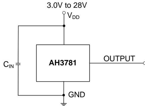
Note: 4.  $C_{IN}$  is for power stabilization and to strengthen the noise immunity, the recommended capacitance is 10nF ~ 100nF.  $R_L$  is the pull-up resistor.
