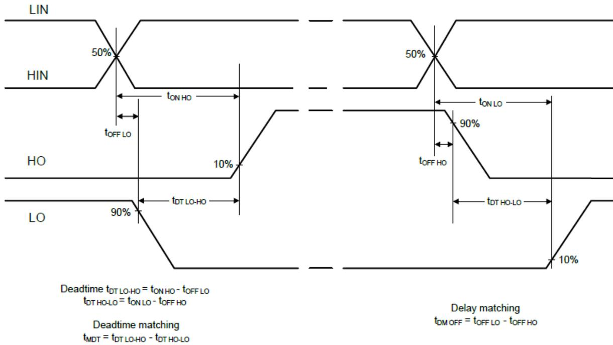
**Figure 2. Switching Time Waveform Definition**
