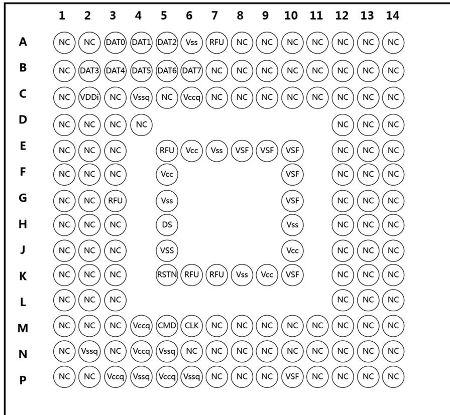
Figure 1. Ball Array (Top View through package)
