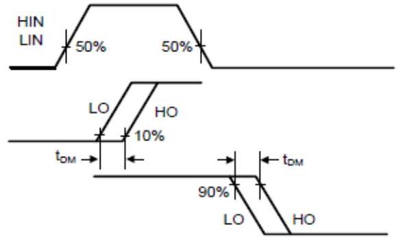
**Figure 2.** Delay Matching Waveform Definitions
