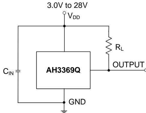
Note: 4.  $C_{IN}$  is for power stabilization and to strengthen the noise immunity, the recommended capacitance is 10nF ~ 100nF.  $R_L$  is the pull-up resistor.
