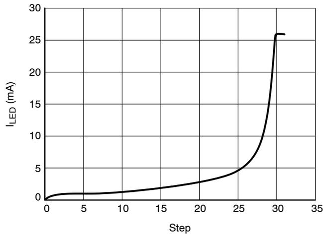
Figure 5. Output Current Programmed Value (ILED = F(Step))
