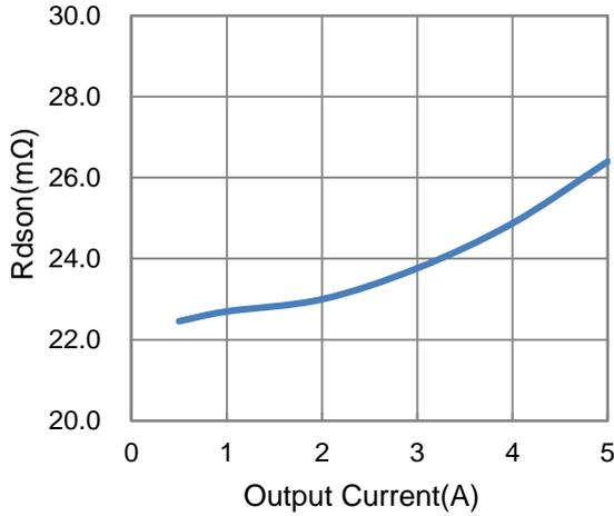
Figure 7 R<sub>ds(on)</sub> vs. Output Current
