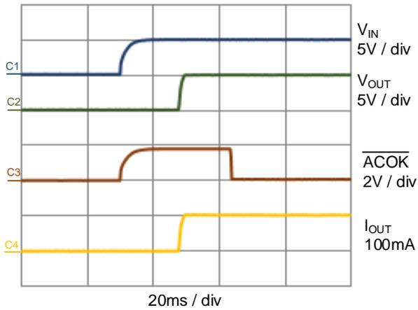
Figure 13 Power-up ( $C_{OUT} = 1\mu F$ , 100mA load).
