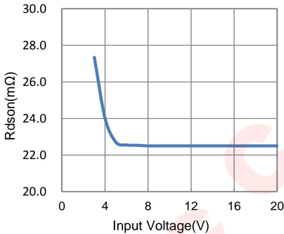
Figure 9 R<sub>ds(on)</sub> vs. Input Voltage (I<sub>out</sub> = 1A)
