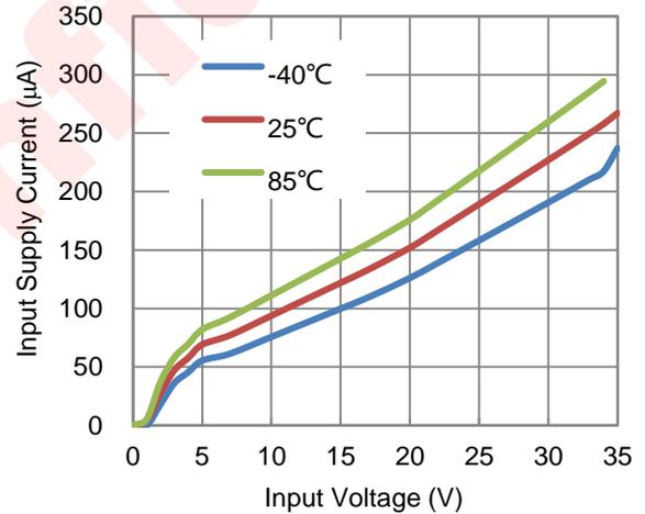
Figure 10 Input Supply Current vs. Supply Voltage
