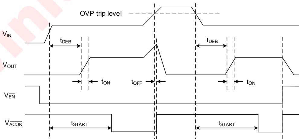
Figure 6 Timing diagram
