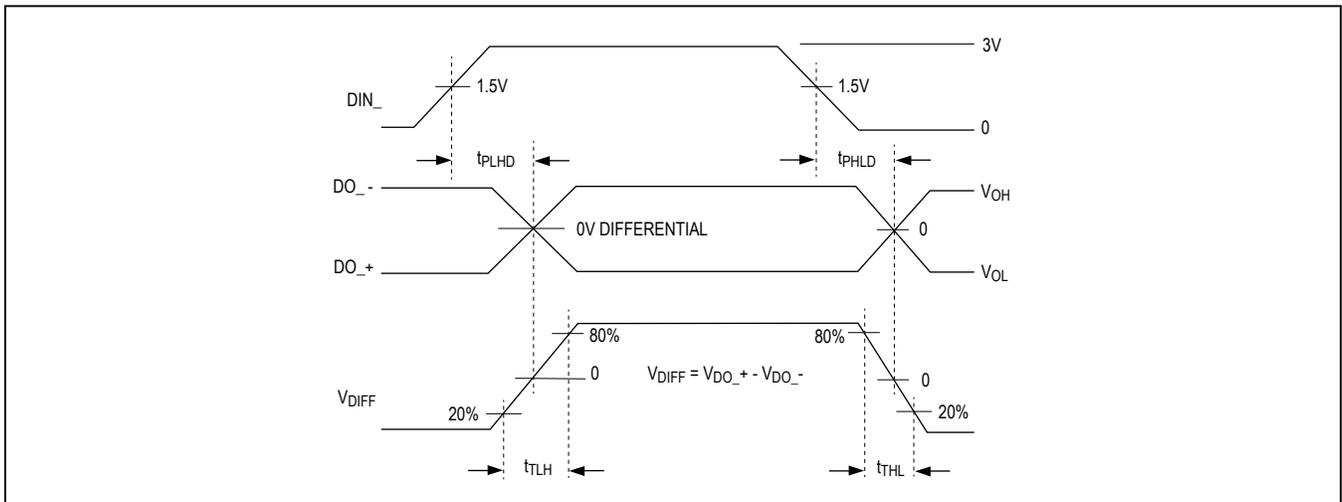
Figure 3. Transmitter Propagation Delay and Transition Time Waveforms
