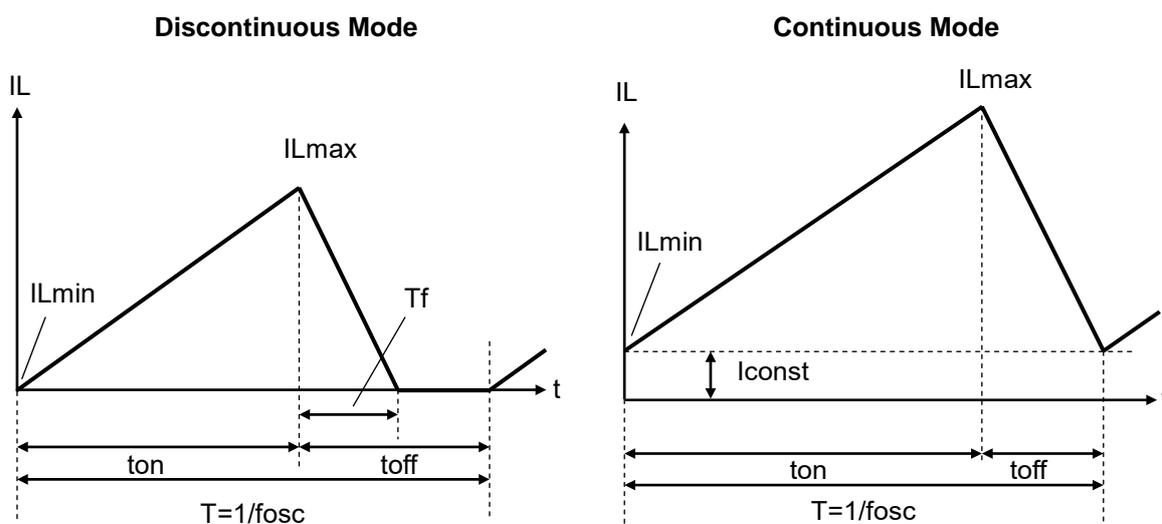
In PWM step-up DC/DC converter, there are two modes; the discontinuous mode and the continuous mode. These two modes depend upon the continuous characteristic of the inductor current.
