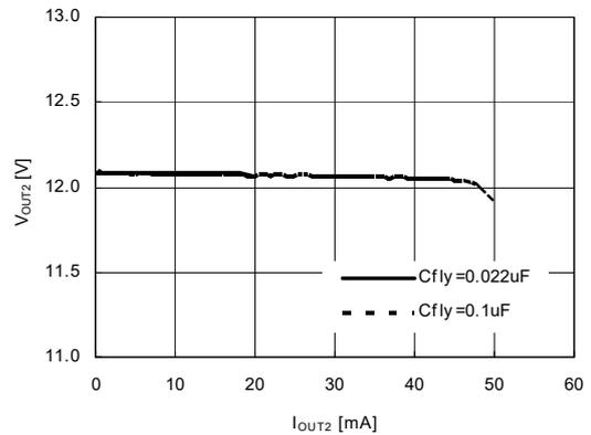
$f_{REQ} = 700\text{kHz}$ ,  $CPVCC = 8.0\text{V}$ ,  $V_{OUT} = 16.0\text{V}$
