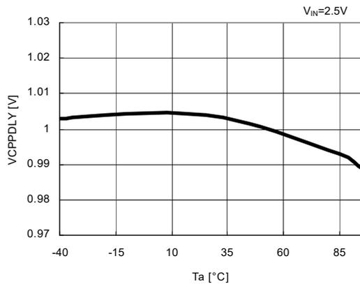
27) CPNDLY Detector Threshold vs. Temperature
