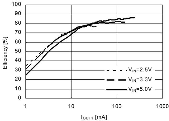
**2)  $V_{OUT2}$  (Step-Up Charge-pump part)**
