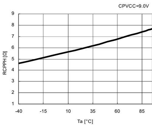
31) CPP<sup>L</sup> ON Resistance vs. Temperature
