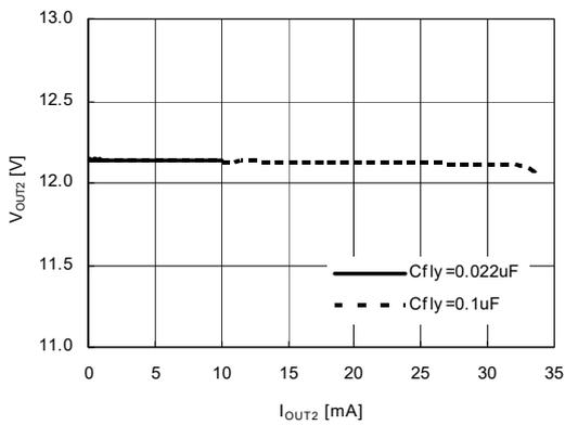
$f_{REQ} = 1400\text{kHz}$ ,  $CPVCC = 8.0\text{V}$ ,  $V_{OUT} = 12.0\text{V}$
