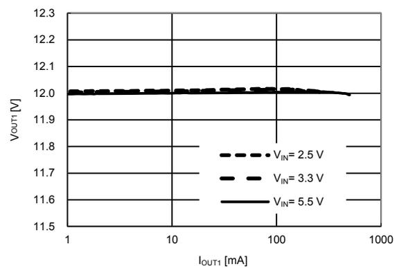
$f_{REQ} = 700\text{kHz}$ ,  $V_{OUT} = 12.0\text{V}$
