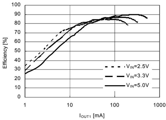
$f_{REQ} = 210kHz, V_{OUT} = 12.0V$
