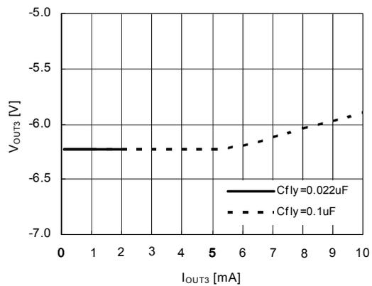
$f_{REQ} = 1400\text{kHz}$ ,  $CPVCC = 8.0\text{V}$ ,  $V_{OUT} = -6.0\text{V}$
