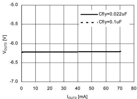
$f_{REQ} = 1400\text{kHz}$ ,  $CPVCC = 12.0\text{V}$ ,  $V_{OUT} = -6.0\text{V}$
