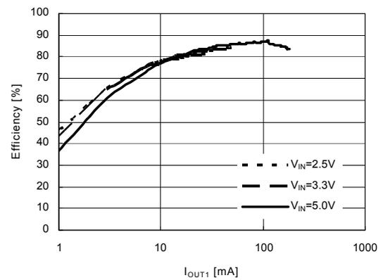
$f_{REQ} = 1400\text{kHz}$ ,  $V_{OUT} = 18.0\text{V}$
