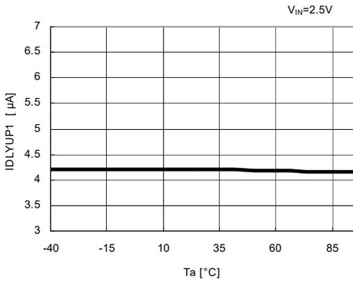
**36) DELAY Discharge Current vs. Temperature**
