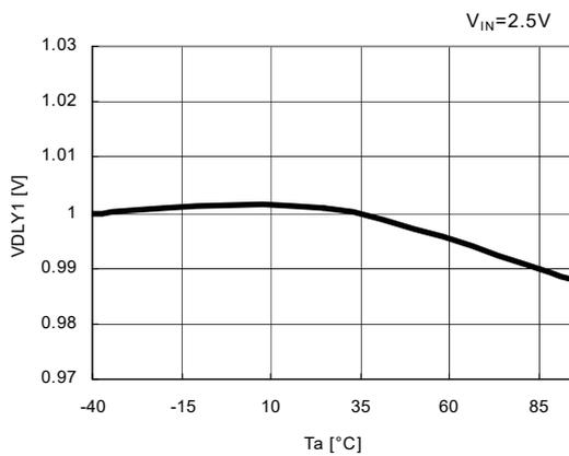
**38) CPPSW "L" Output Voltage vs. Temperature**
