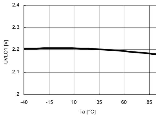
11) UVLO Release Voltage vs. Temperature
