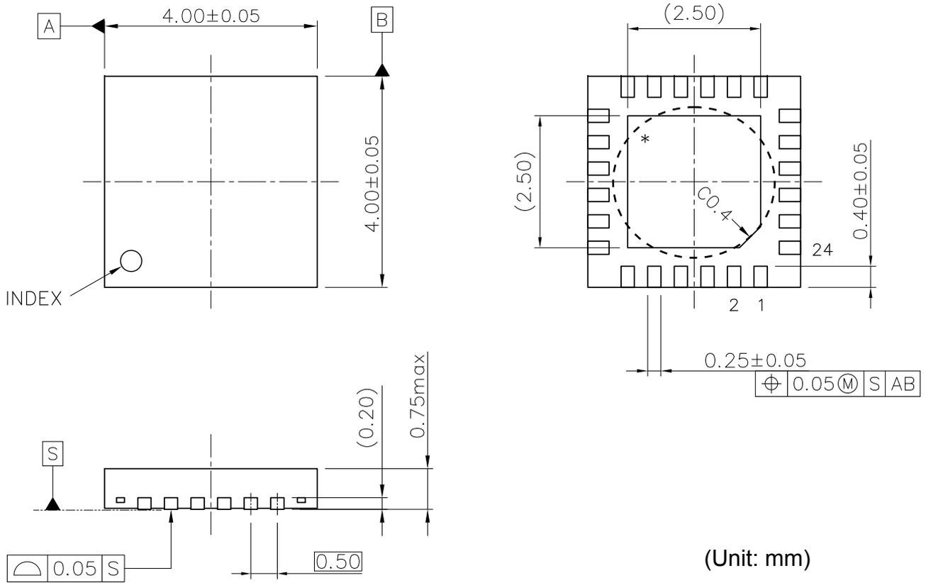
\* The tab on the bottom of the package enhances thermal performance and is electrically connected to GND (substrate level). The tab is recommended to connect to the ground plane on the board. Otherwise it may be left floating.
