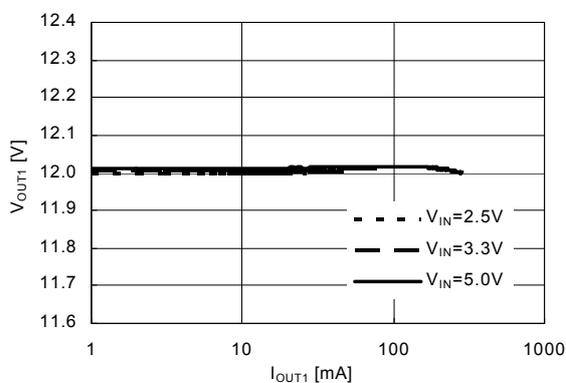
$f_{REQ} = 1400\text{kHz}$ ,  $V_{OUT} = 12.0\text{V}$
