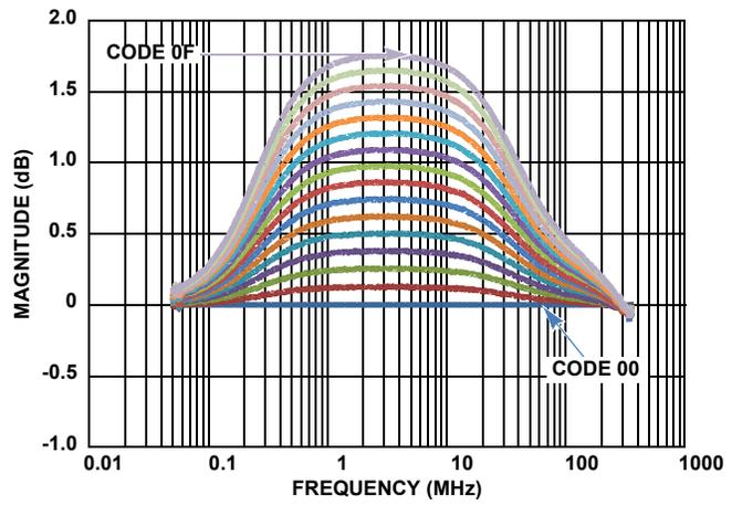
FIGURE 9. FREQUENCY RESPONSE vs 200kHz BITS 3:0
