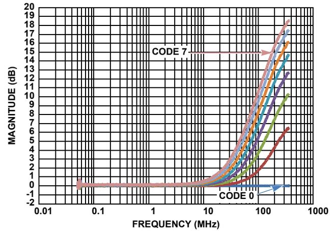
FIGURE 5. FREQUENCY RESPONSE vs 100MHz BITS 7:5
