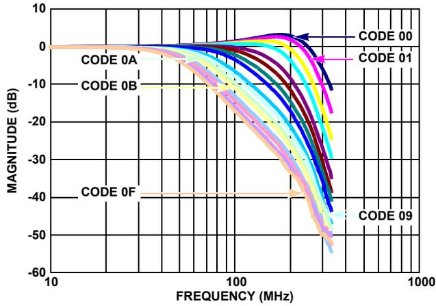
FIGURE 10. FREQUENCY RESPONSE vs LOW PASS FILTER BITS 3:0
