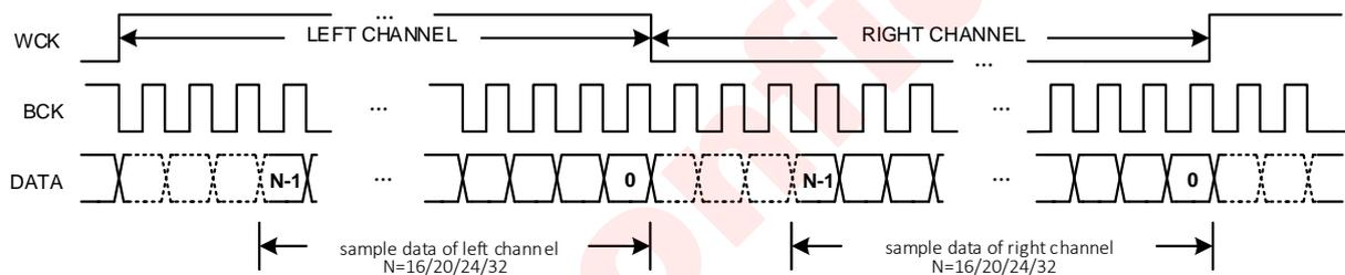
**Figure 11 I<sup>2</sup>S Timing for Right-Justified Mode**
