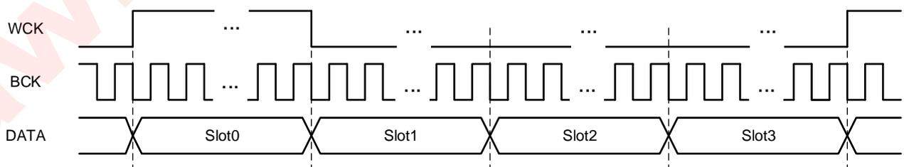
**Figure 12 TDM Timing**
