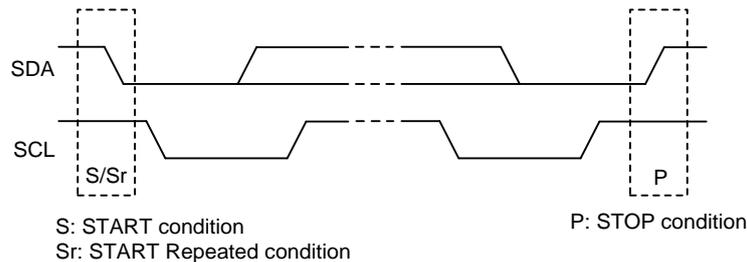
Figure 16 I<sup>2</sup>C Start/Stop Condition Timing
