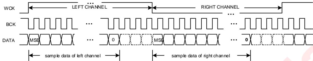
**Figure 10 I<sup>2</sup>S Timing for Left-Justified Mode**
