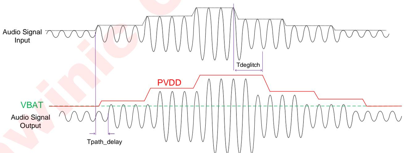
Figure 14 Boost Circuit Behavior in Smart Boost 2 Mode
