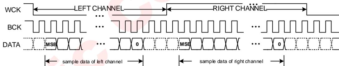
**Figure 9 I<sup>2</sup>S Timing for Standard I<sup>2</sup>S Mode**
