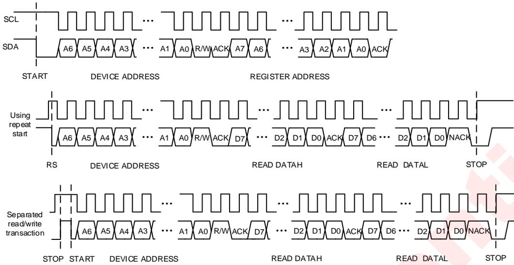
Figure 19 I<sup>2</sup>C Read Byte Cycle
