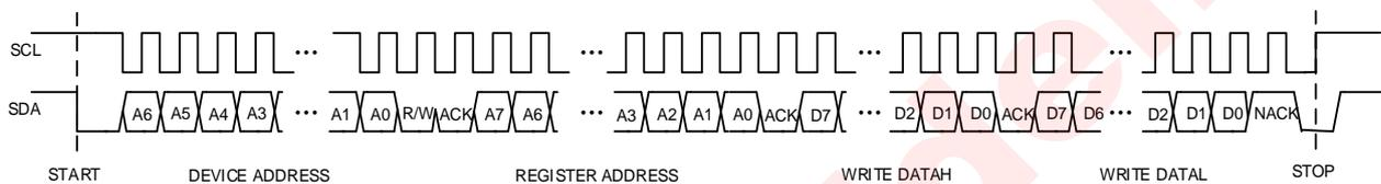
Figure 18 I<sup>2</sup>C Write Byte Cycle
