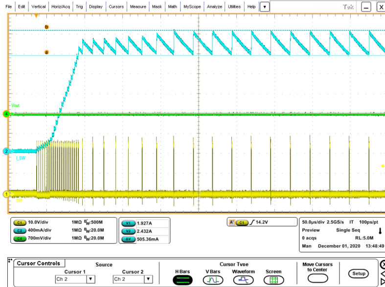
Figure 22. Soft-start procedure with V_{OUT} shorted to GND
