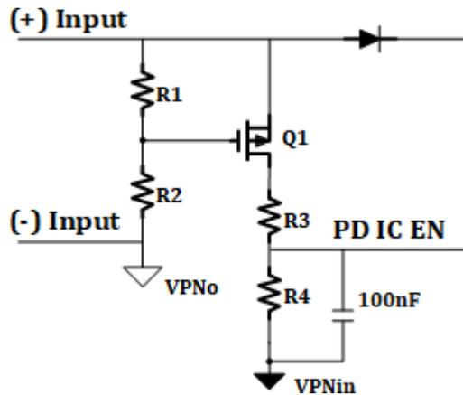
R1 and R2 set a rough threshold for PFET Q1 enable, to detect whether the external adapter exists or not. It must be set at a lower threshold than the PD70211 disable levels.
