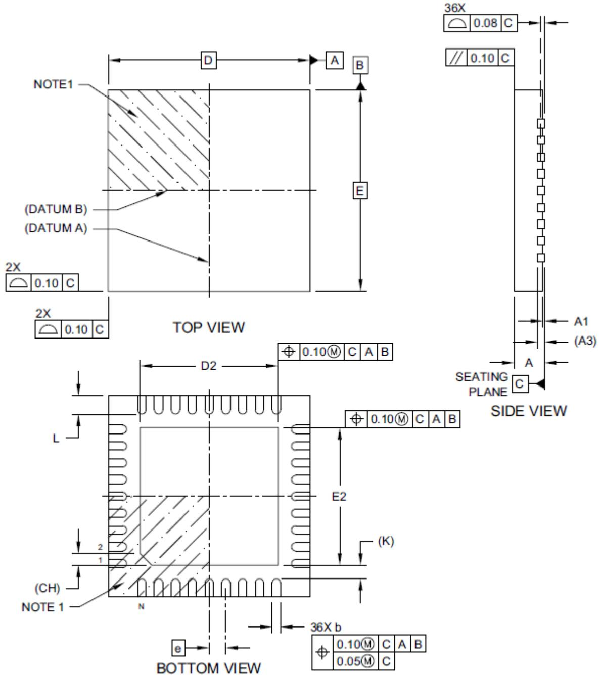
**Note:** Dimensions do not include protrusions; they must not exceed 0.155 mm (0.006") on any side. Lead dimension does not include solder coverage.
