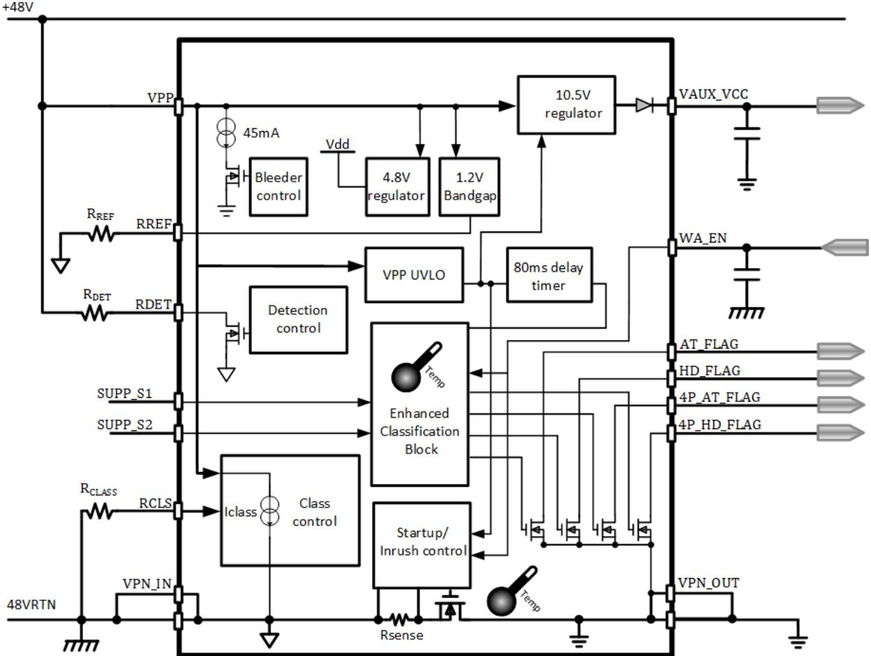
Figure 1-2. PD70211 Block Diagram (PWM Section)
