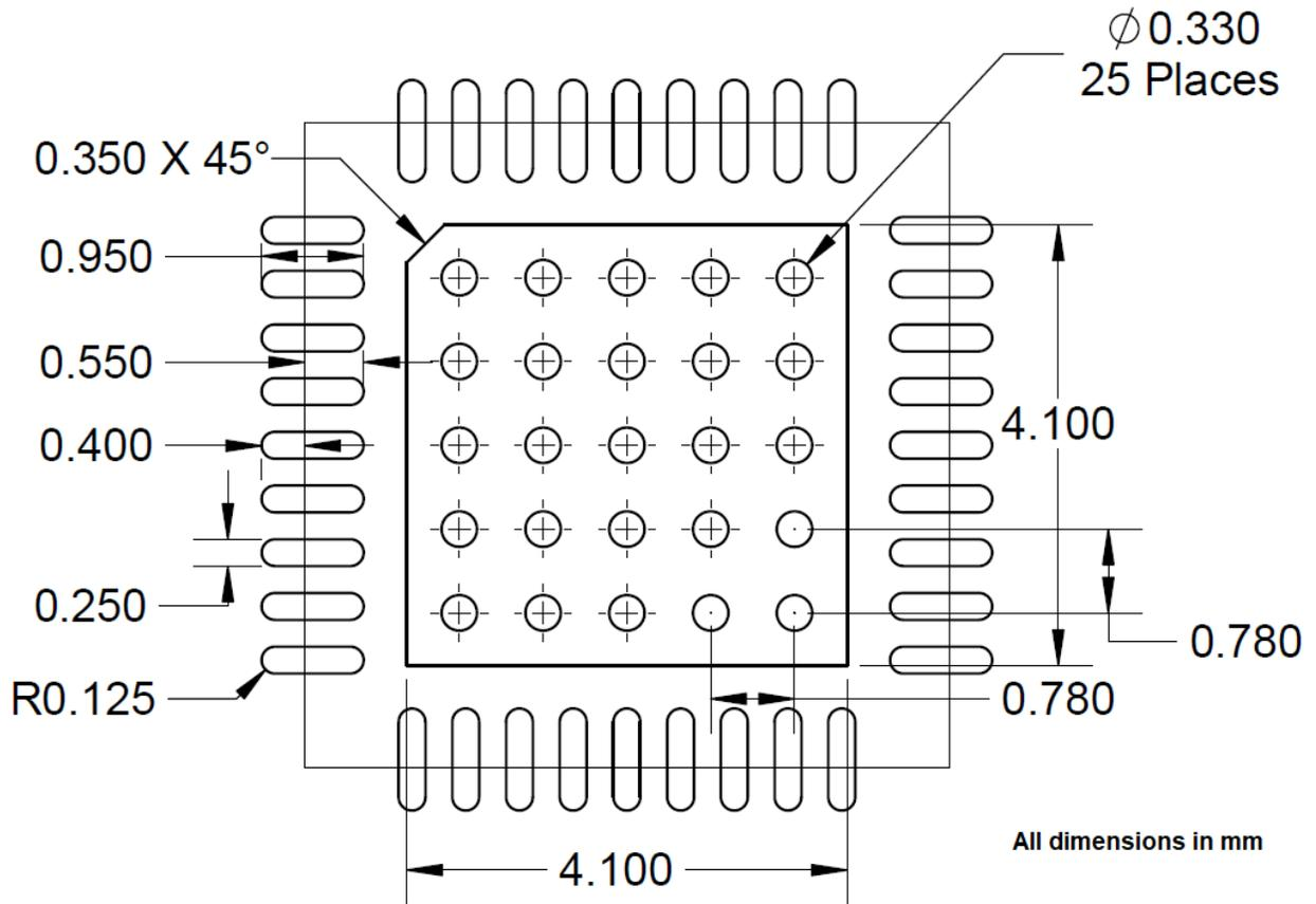
Figure 4-4. Paste Mask (Top View)
