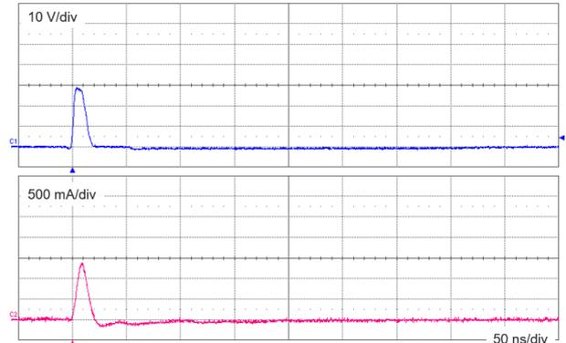
**Figure 10. ISO7637-3, slow transient pulse - negative 2a ( $U_s = -85\text{ V}$ )**
