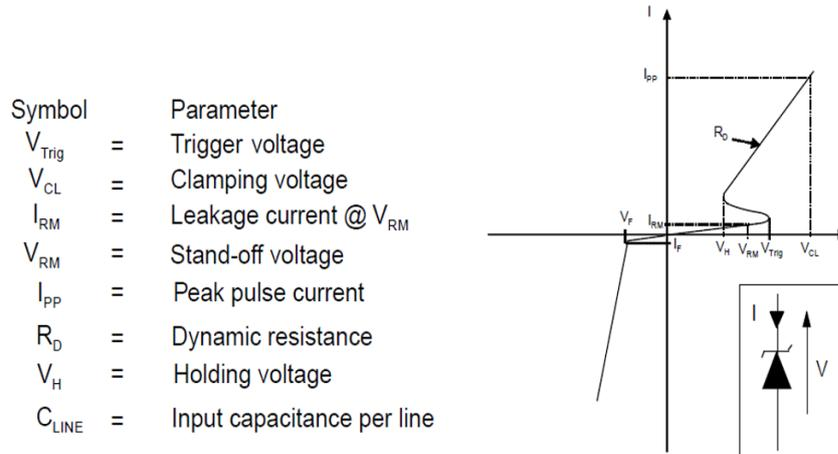
**Table 2. Electrical characteristics (values) ( $T_{amb} = 25^{\circ}C$ )**
