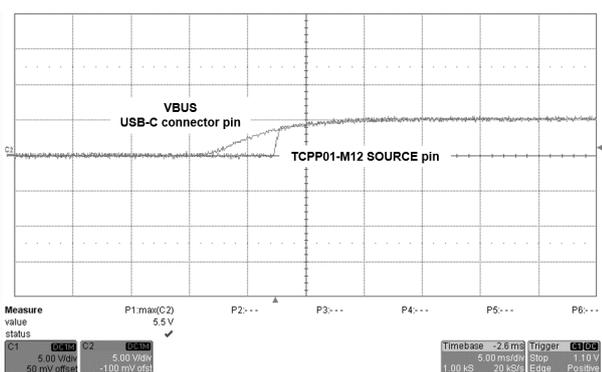
Figure 16. VBUS 5 V overvoltage protection (sink configuration, 20 V applied on VBUS)
