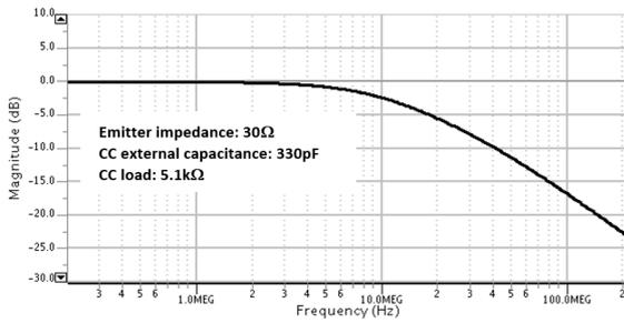
Figure 6. CC line bandwidth:  $V_{cm} = 1.2\text{ V}$
