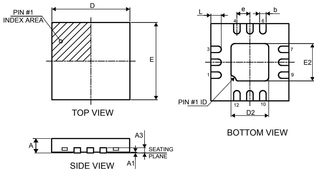
Table 16. QFN-12L package mechanical data
