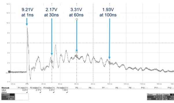
Figure 14. CCx line TLP curve (unpowered)
