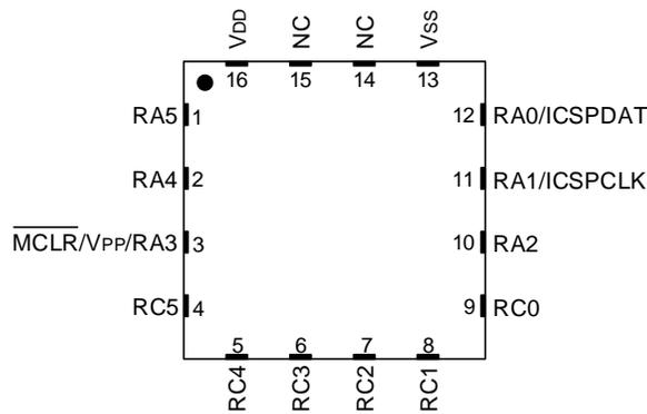
**Note:** It is recommended that the exposed bottom pad be connected to  $V_{SS}$ , however, it must not be the only  $V_{SS}$  connection to the device.
