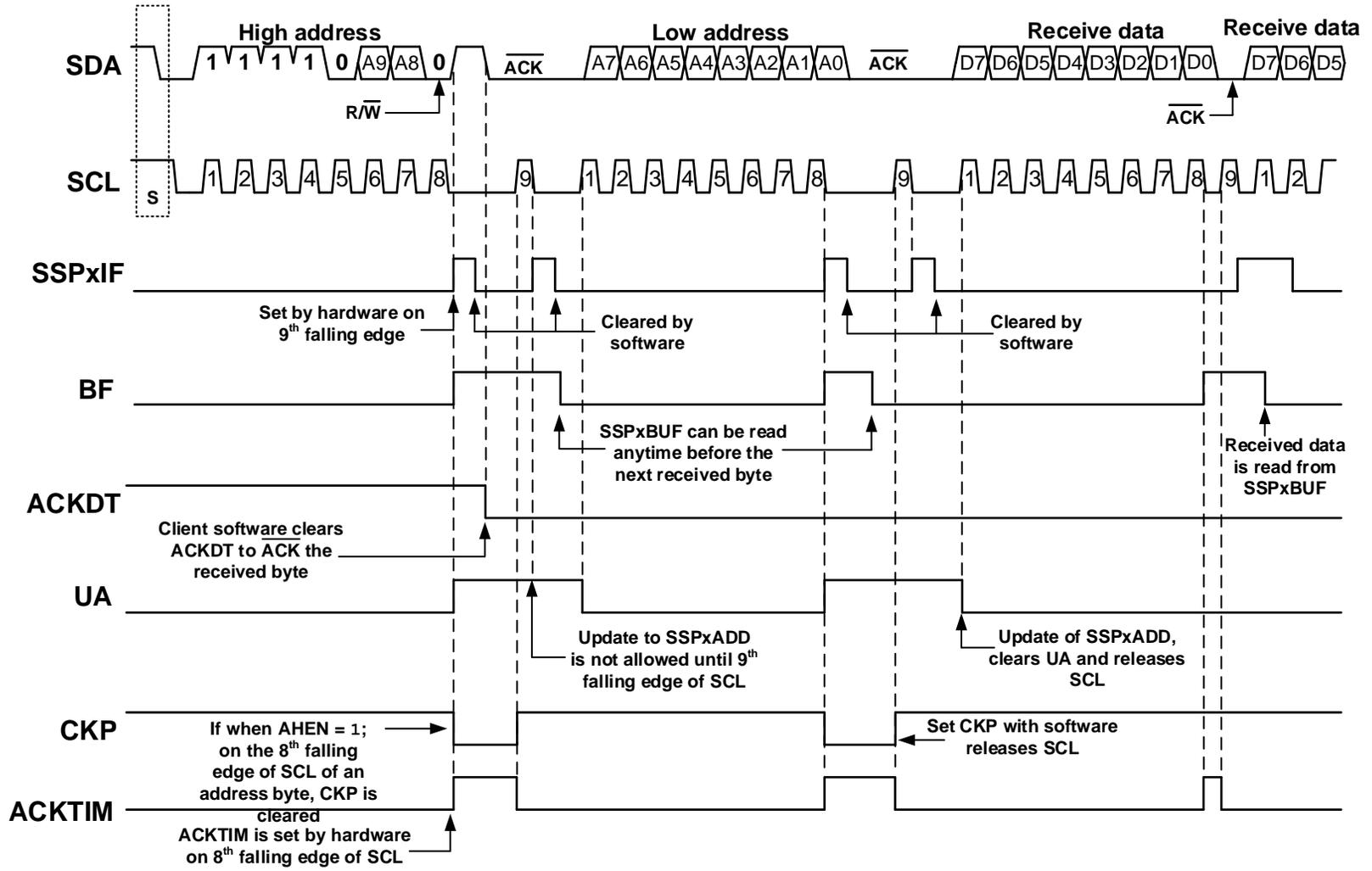
**Figure 29-21. I<sup>2</sup>C Client, 10-Bit Address, Transmission (SEN = 0, AHEN = 0, DHEN = 0)**
