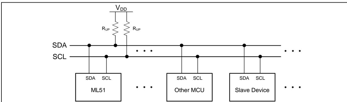
Figure 6.11-1 I<sup>2</sup>C Bus Interconnection
