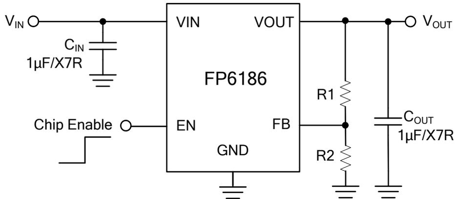
Figure 2. Typical Application Circuit for FP6186 adjustable voltage
