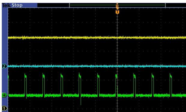
Fig 5.  $V_{IN} = 100V$ ,  $V_{OUT} = \text{short to GND}$
