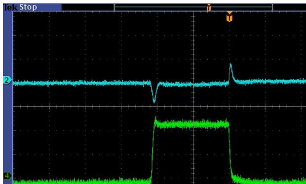
Fig 3. Load transient 0 to 50mA
