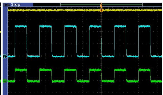
Fig 6.  $V_{IN}=36V$ ,  $V_{OUT}=5V$ ,  $R_{LOAD}= 100 \text{ ohm}$ , thermal protect
