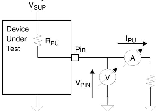
Figure 7. Internal Resistor Test Conditions,  $T_A = 0^{\circ}\text{C}$  to  $70^{\circ}\text{C}$
