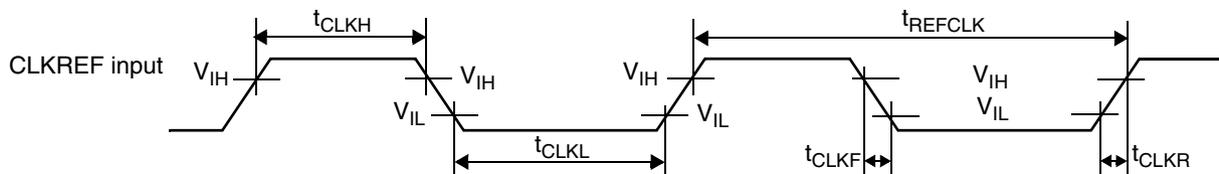
Figure 13. CLKREF Clock Waveforms
