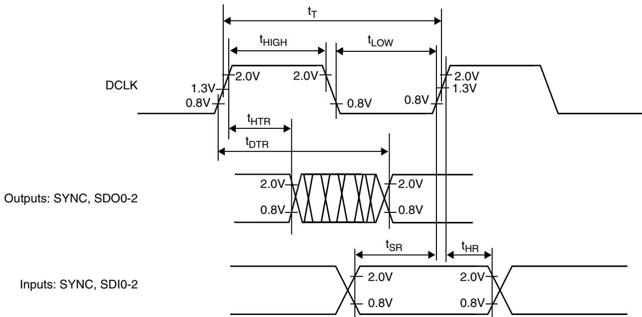
Figure 18. SSI Signal Timing
