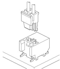
This SFV connector is a wire-to-board connector for connecting power supply and PCB and withstands high voltage. It is used for power supply of LED backlight in Liquid Crystal Display Television set.
