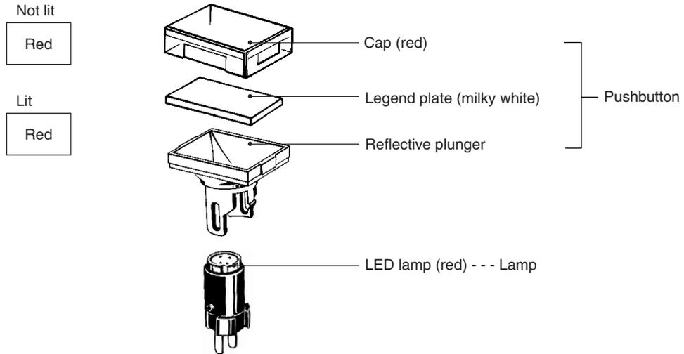
"Colored illumination" describes LED models for which the screen color is white when the LED is not lit and changes to the color of the LED lamp when the LED is lit.
