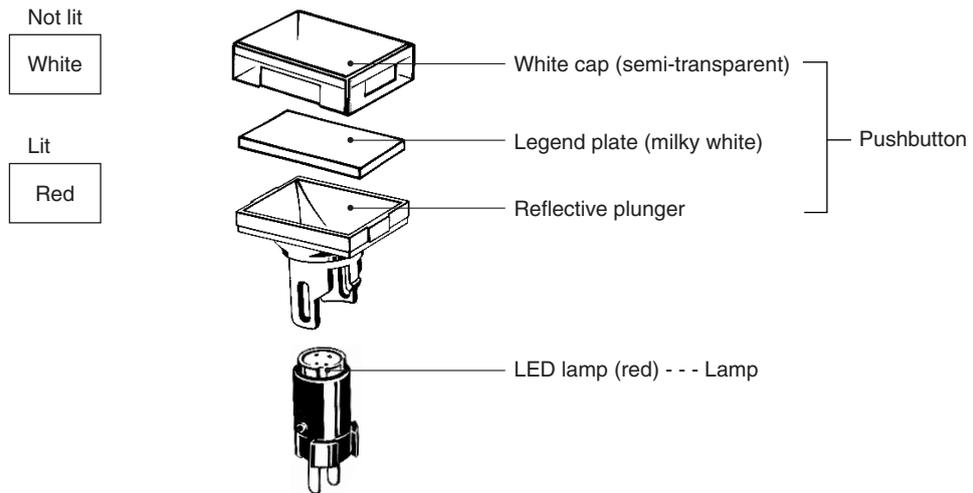
**Ordering: With colored-illumination models, order the Pushbutton, Lamp, and Switch as shown in the following table.**
