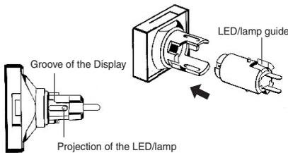
Note: Push the projections on the Lamp into the grooves on the Pushbutton/Display. The Lamp for Lighted Pushbutton Switches moves, but the Lamp for Indicators is fixed.
