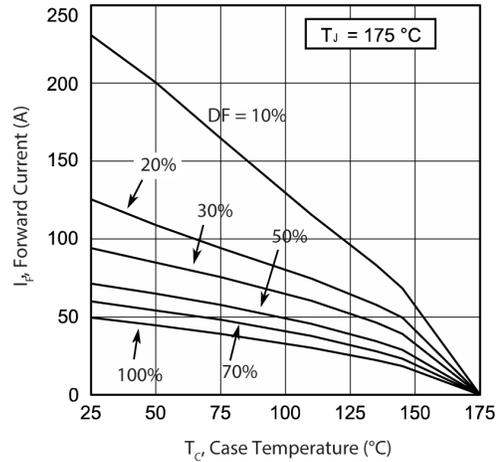
Figure 3 • Max. Forward Current vs. Case Temp.
