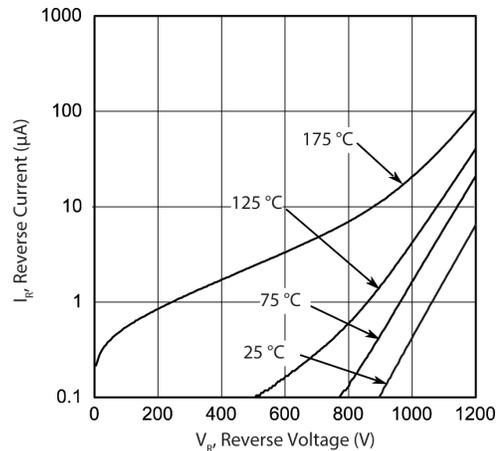
Figure 5 • Reverse Current vs. Reverse Voltage
