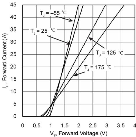
Figure 2 • Forward Current vs. Forward Voltage
