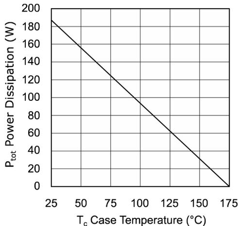
Figure 4 • Max. Power Dissipation vs. Case Temp.
