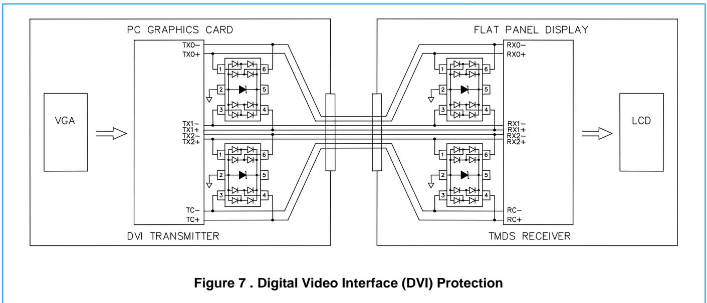
Figure 7 . Digital Video Interface (DVI) Protection
