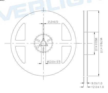
**Note:** The tolerances unless mentioned are  $\pm 0.1$ mm, unit = mm.
