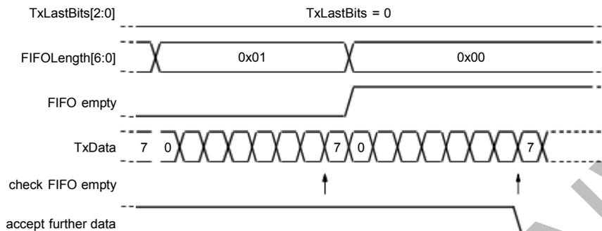
**Fig 13. Timing for transmitting byte oriented frames**
