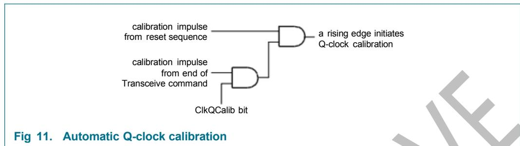
Fig 11. Automatic Q-clock calibration
