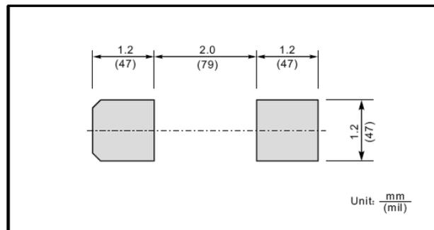
• Recommended condition of flow soldering
