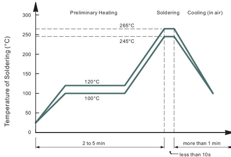
• Recommended condition of reflow soldering
