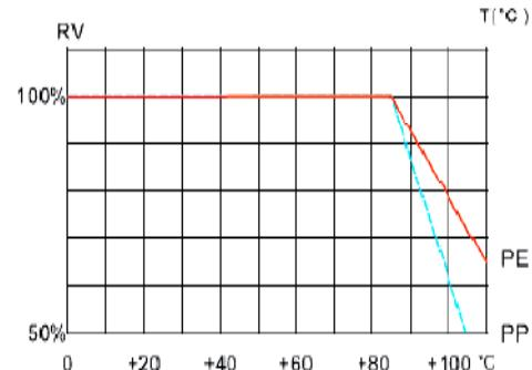
注: 电容器工作电压 (Operating voltage of the capacitor)
