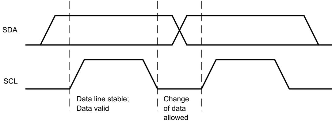
图 9-9. Bit Transfer on the I<sup>2</sup>C Bus
