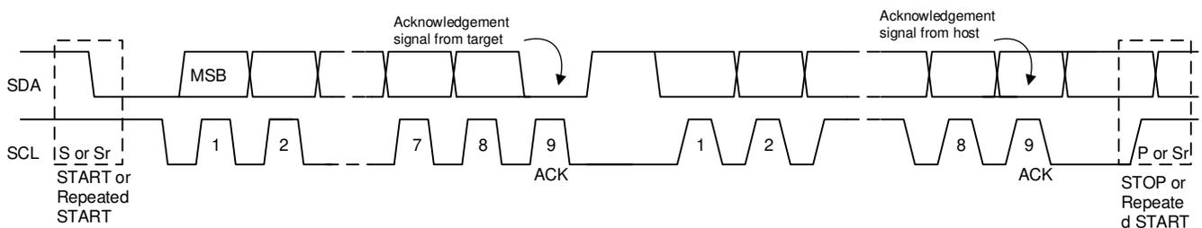
图 9-11. Data Transfer on the I<sup>2</sup>C Bus
