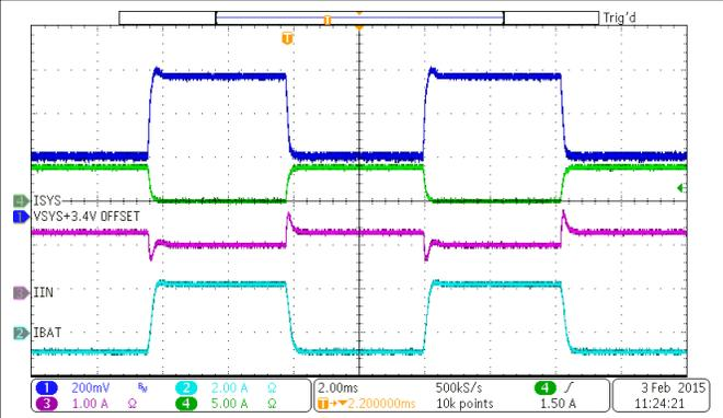
VBUS = 9 V I<sub>CHG</sub> = 2 A I<sub>IN</sub> = 1.5 A VBAT = 3.8 V
