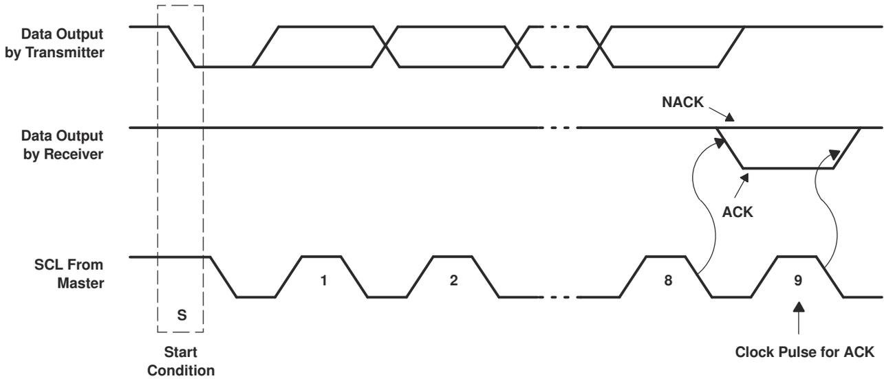
**图 8-4. Acknowledgment on the I<sup>2</sup>C Bus**
