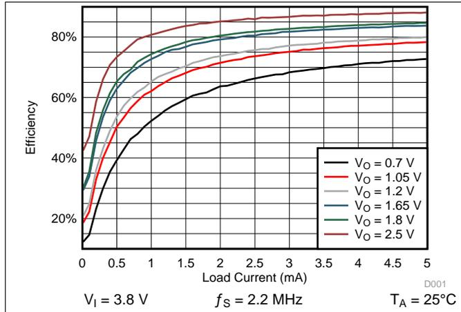
图 4-4. SMPS Efficiency for all SMPS in Eco-mode
