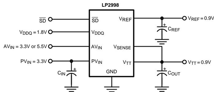
**Figure 22. DDR-II Termination with Higher Voltage Rails**
