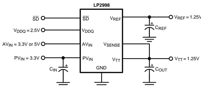
Figure 25. SSTL-2 Implementation with Higher Voltage Rails
