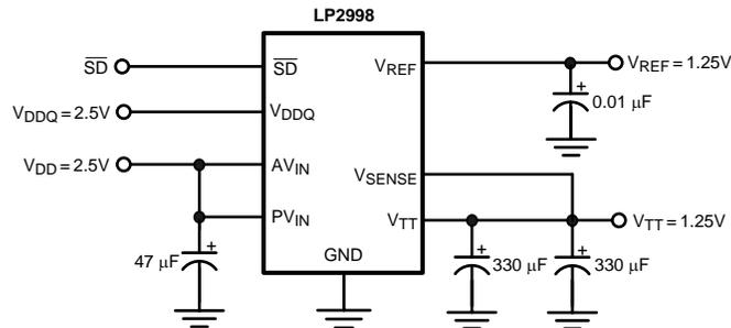
Figure 29. Typical SSTL-2 Application Circuit for Motherboards
