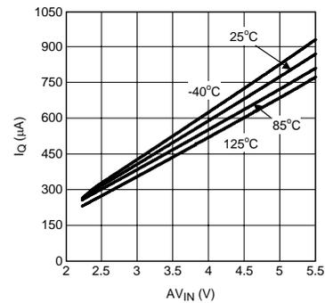
Figure 8.  $I_Q$  vs  $AV_{IN}$  Over Temperature
