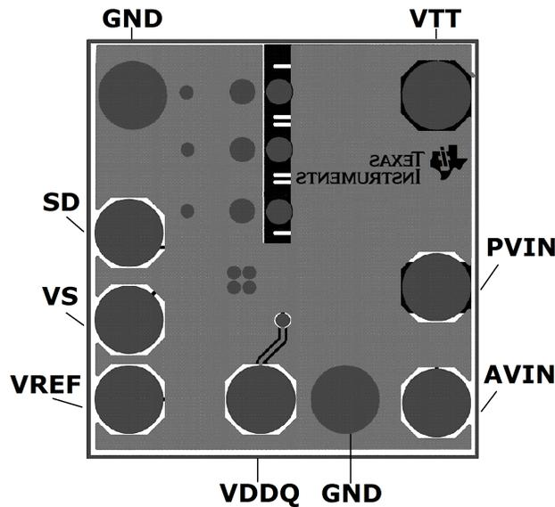
Figure 32. LP2998EVM SO PowerPAD Layout Example (Back)
