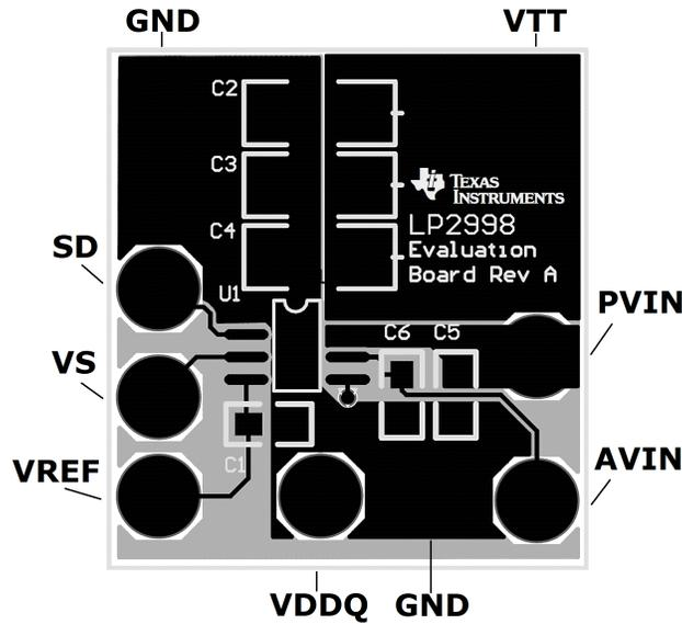
Figure 31. LP2998EVM SO PowerPAD Layout Example (Front)
