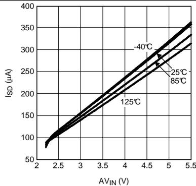
Figure 7.  $I_{SD}$  vs  $AV_{IN}$  Over Temperature
