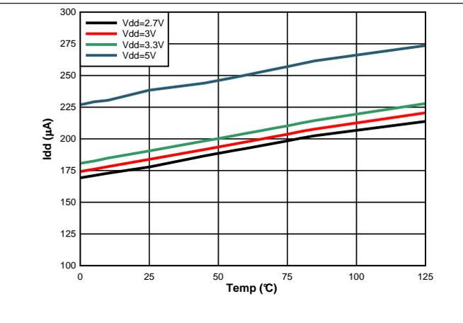
Figure 5. Supply Current vs. Temperature, RH Measurement Active
