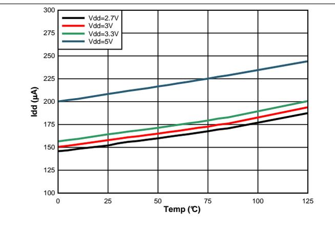
Figure 7. Supply Current vs. Temperature, Temp Measurement Active
