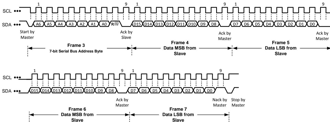
Figure 14. Read Humidity and Temperature Measurement (Data Ready)
