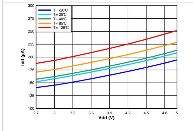
Figure 6. Supply Current vs. Supply Voltage, Temp Measurement Active
