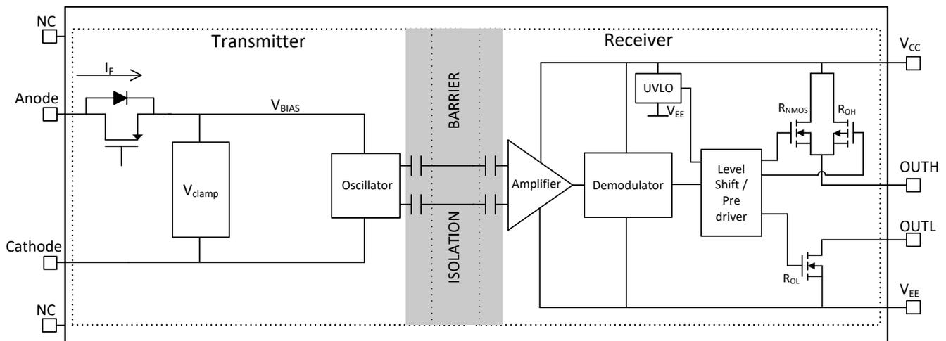
**Figure 8-3. Functional Block Diagram for UCC23514S (Split output)**
