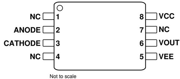
**Figure 5-4. UCC23514V DWV Package 8-pin SOIC-WB Top View**
