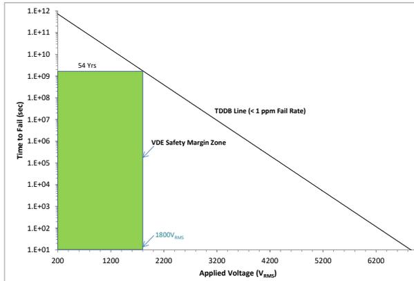
Figure 6-1. Reinforced Isolation Capacitor Life Time Projection
