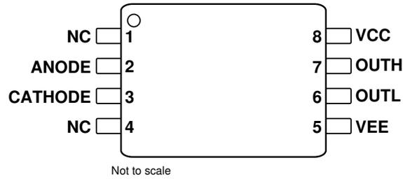
**Figure 5-3. UCC23514S DWV Package 8-pin SOIC-WB Top View**
