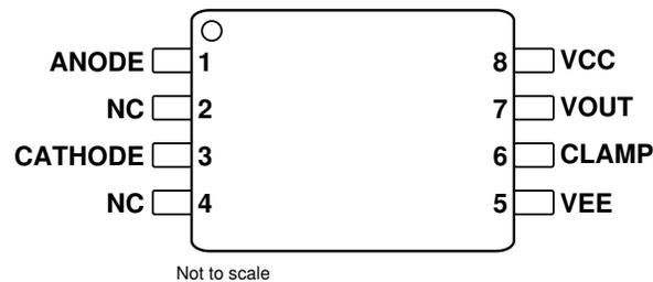
Figure 5-2. UCC23514M DWV Package 8-pin SOIC-WB Top View
