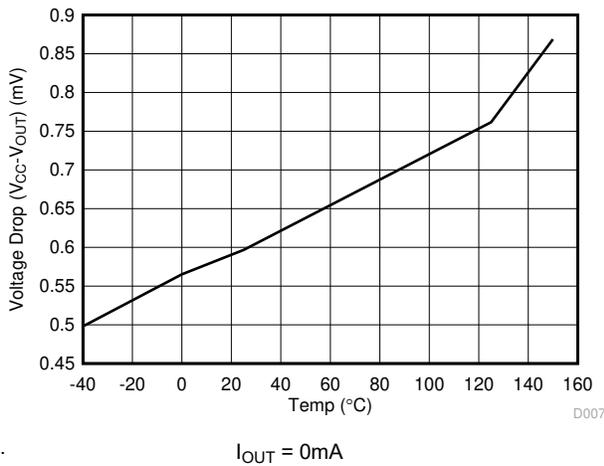
A. **Figure 6-8. V<sub>OH</sub> (No Load) versus Temperature**
