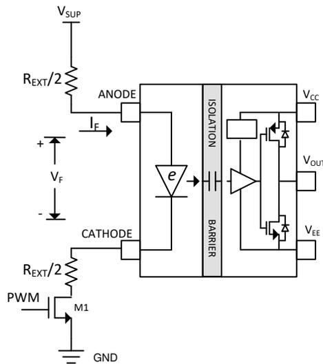
$$R_{EXT} = \frac{V_{SUP} - V_F}{I_F} - R_{M1}$$
