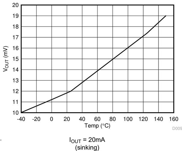
A. **Figure 6-10. V<sub>OL</sub> versus Temperature**
