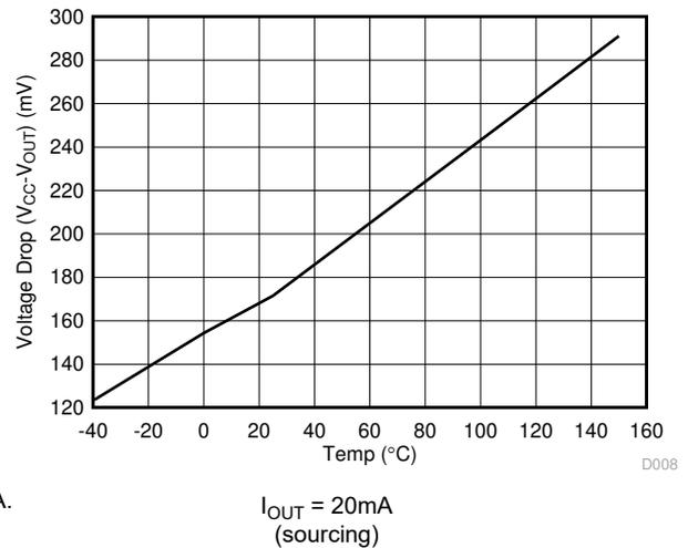
A. **Figure 6-9. V<sub>OH</sub> (20mA Load) versus Temperature**
