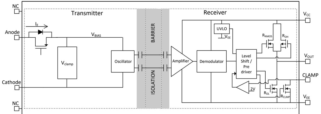
**Figure 8-2. Functional Block Diagram for UCC23514M (Miller clamp)**
