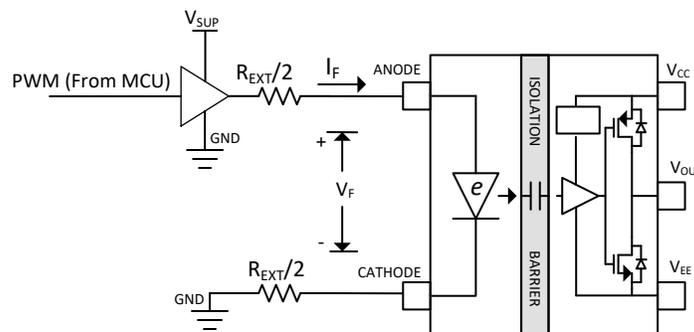
$$R_{EXT} = \frac{V_{SUP} - V_F}{I_F} - R_{OH\_buf}$$
