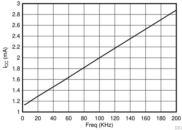
**Figure 6-12. Supply current versus Frequency**
