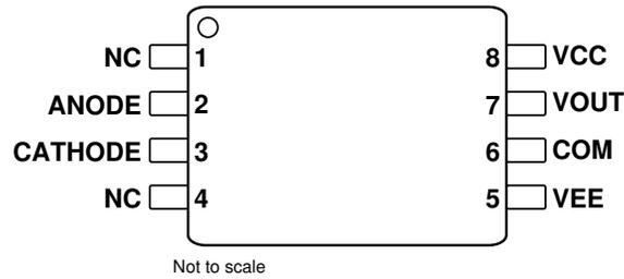
Figure 5-1. UCC23514E DWV Package 8-pin SOIC-WB Top View
