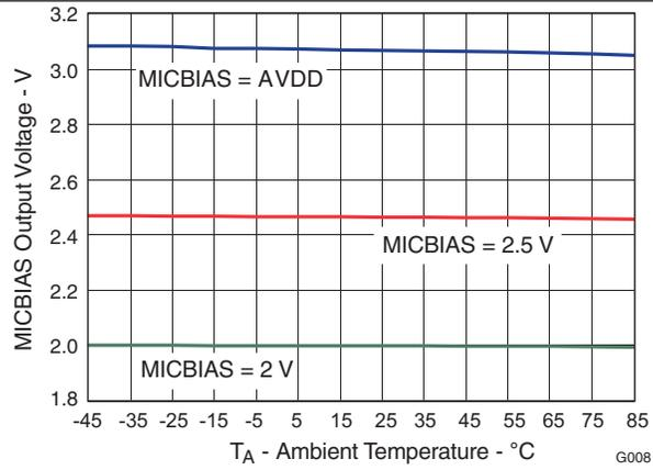
图 11. MICBIAS Output Voltage vs Ambient Temperature
