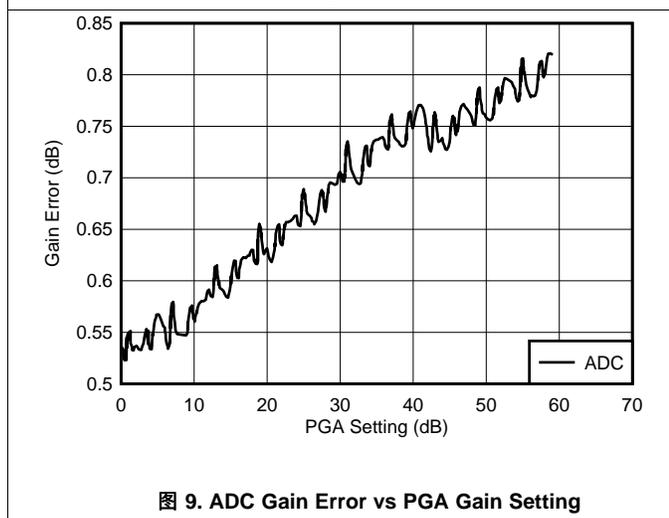
图 9. ADC Gain Error vs PGA Gain Setting
