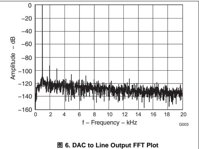
图 6. DAC to Line Output FFT Plot
