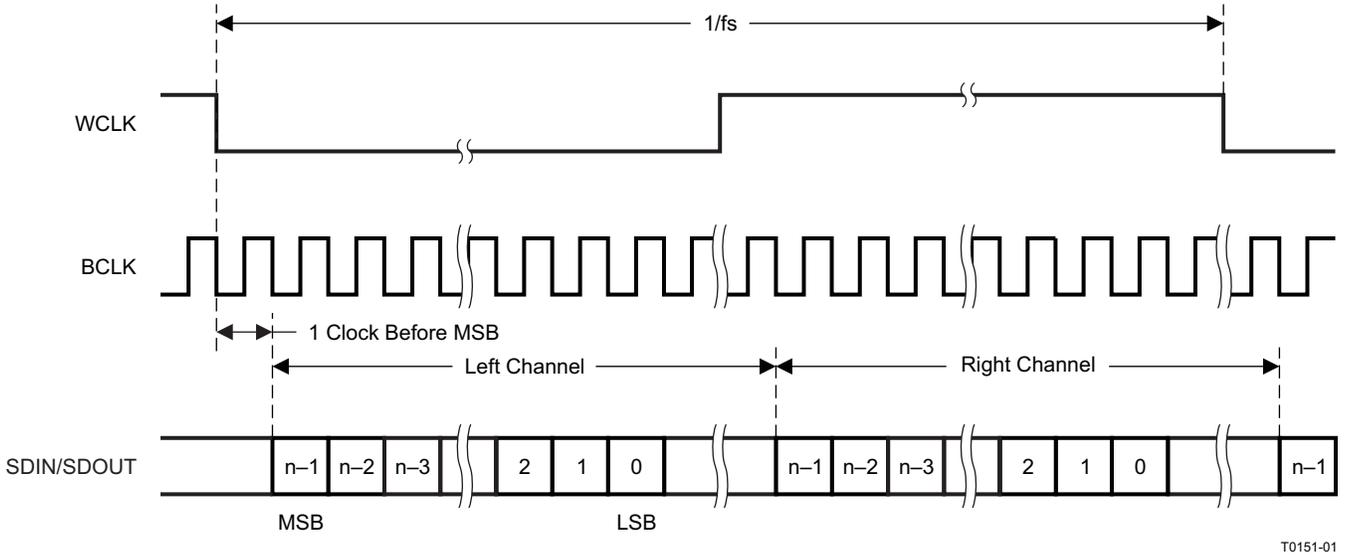
图 14. I<sup>2</sup>S Serial Data Bus Mode Operation
