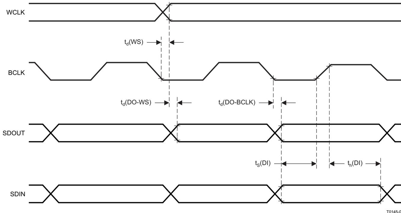
图 1. I<sup>2</sup>S, Left-Justified and Right-Justified Format Timing in Master Mode
