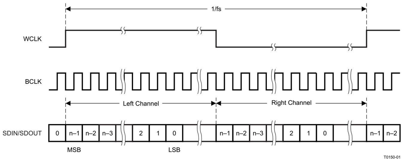
图 13. Left-Justified Serial Data Bus Mode Operation
