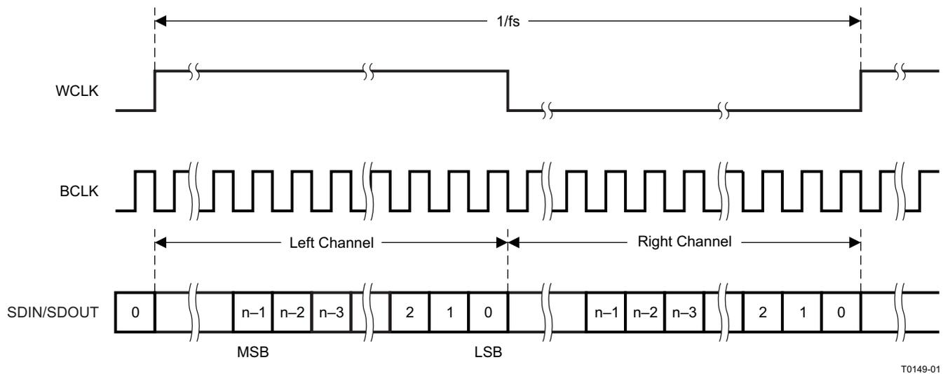
图 12. Right-Justified Serial Data Bus Mode Operation
