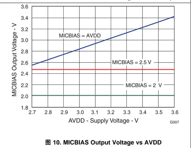
图 10. MICBIAS Output Voltage vs AVDD
