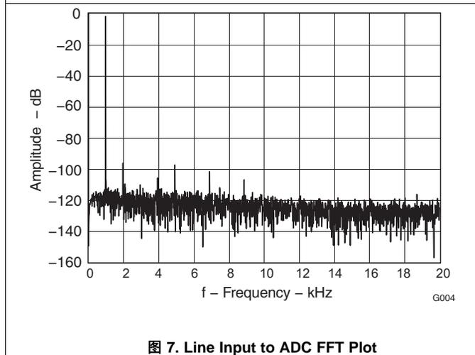
图 7. Line Input to ADC FFT Plot
