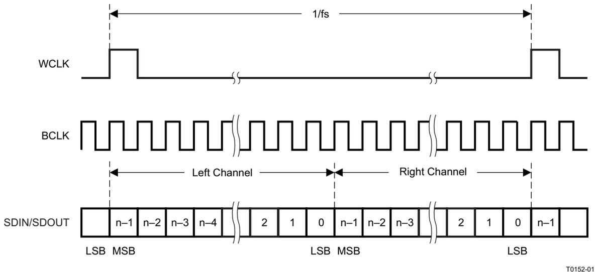
图 15. DSP Serial Data Bus Mode Operation
