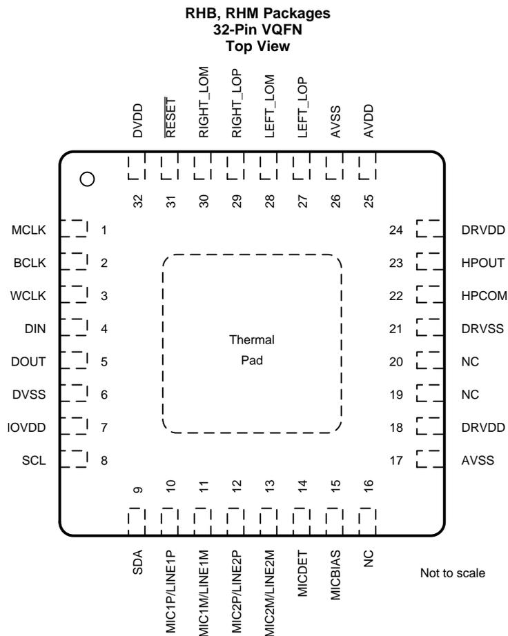
NOTE: Connect the device thermal pad to DRVSS.
