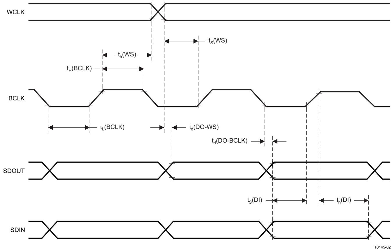
图 3. I<sup>2</sup>S, Left-Justified and Right-Justified Format Timing in Slave Mode
