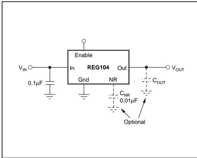
FIGURE 1. Fixed Voltage Nominal Circuit for REG104.
