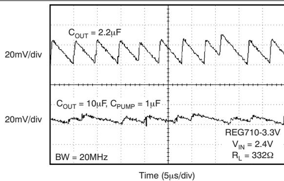
Figure 16. Output Ripple Voltage
