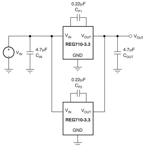
**Figure 22. REG710 Circuit for Doubling the Output Current**
