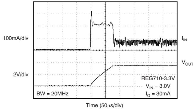
Figure 20. Input Current at Turn-On
