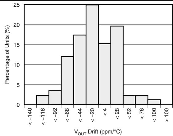
Figure 4. Output Voltage Drift Histogram
