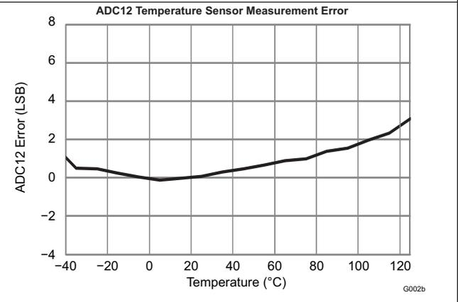
Figure 7. ADC12 Temperature Sensor Measurement Error vs. Temperature
