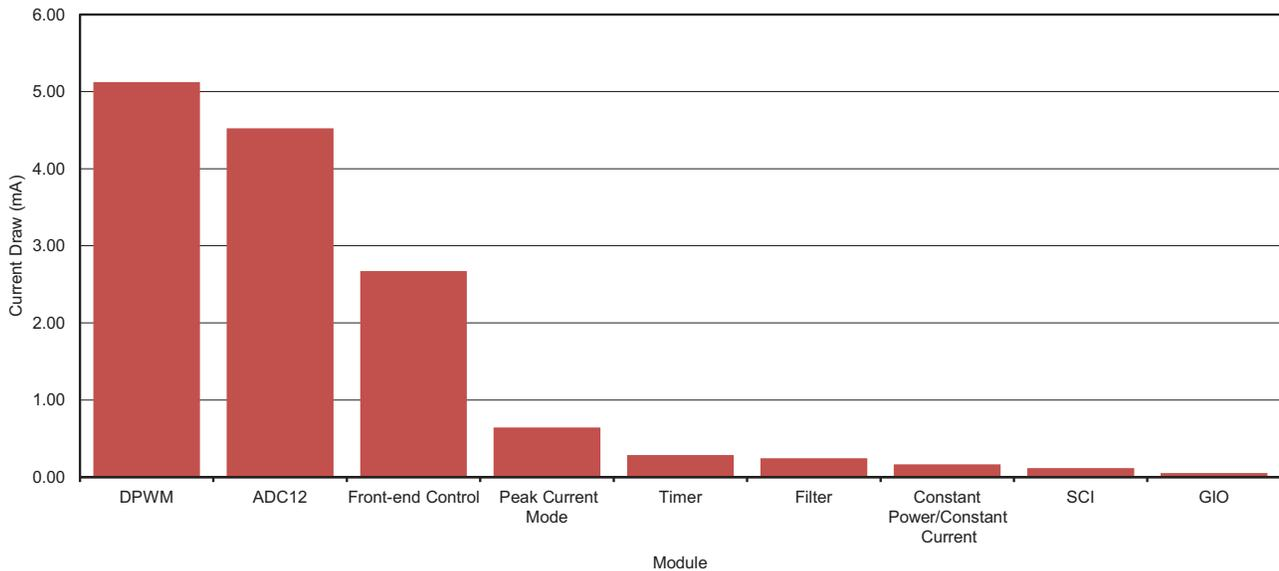
The CLKGATECTRL register provides control bits that can enable or disable the clock to several peripherals such as, PCM, CPCC, digital filters, front ends, DPWMs, UARTs, ADC-12 and more.
