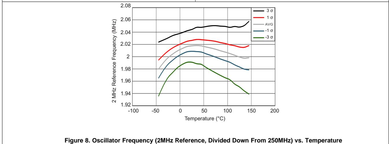
Figure 8. Oscillator Frequency (2MHz Reference, Divided Down From 250MHz) vs. Temperature
