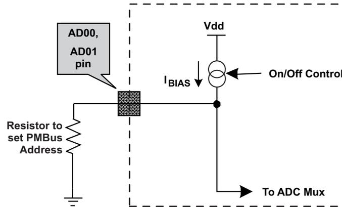
Figure 24. PMBUS Address Detection Method
