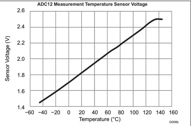
Figure 5. ADC12 Measurement Temperature Sensor Voltage vs. Temperature
