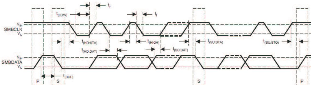
**Figure 1. IC/SMBUS/PMBUS Timing Diagram<sup>2</sup>**
