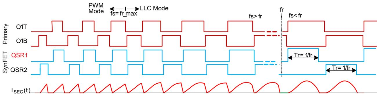
Figure 13. LLC Waveforms
