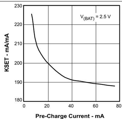
Figure 6. KSET Linearity vs Pre-Charge Current
