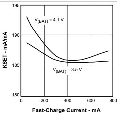
Figure 5. KSET Linearity vs Fast-Charge Current
