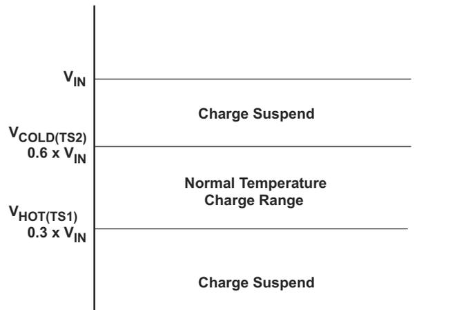
Figure 11. Battery Temperature Qualification With NTC Thermistor
