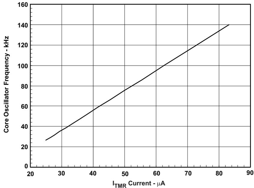
Figure 14. bq24085/6/7/8 Oscillator Linearity vs I<sub>TMR</sub>
