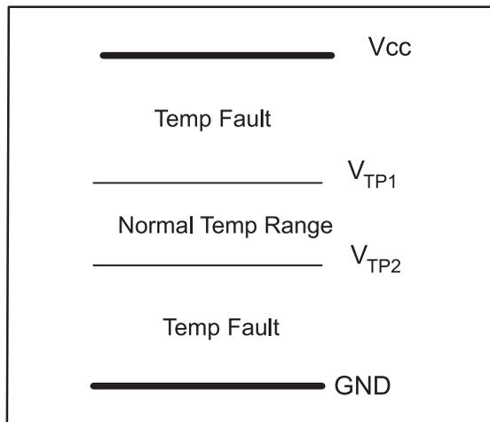
Figure 17. Temperature Threshold
