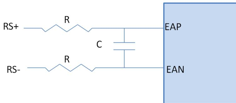
图 12-5. Local Filter on EAPx and EANx Pins
