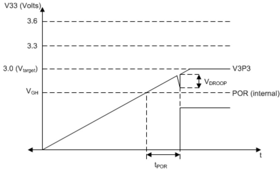
图 11-1. V33 Voltage Dip When POR is Activated
