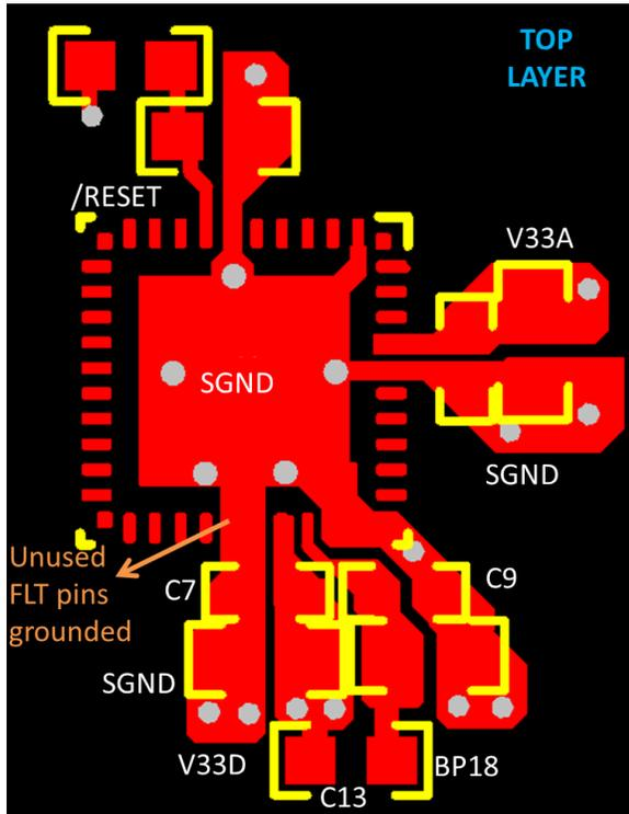
图 12-10. UCD3138 and UCD3138064 40 Pin Layout Top Layer
