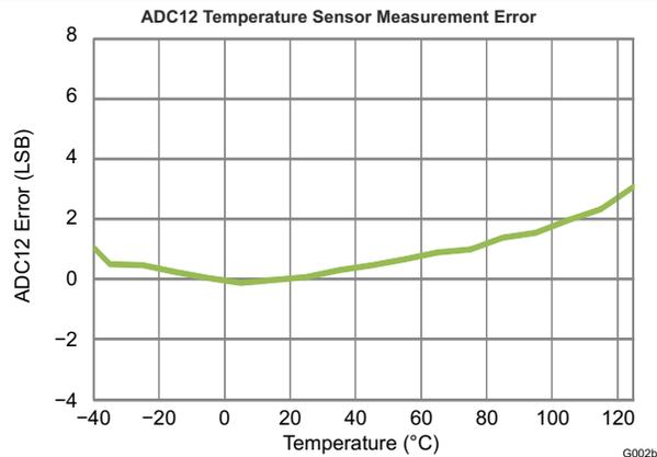
**图 8-11. ADC12 Temperature Sensor Measurement Error vs Temperature**
