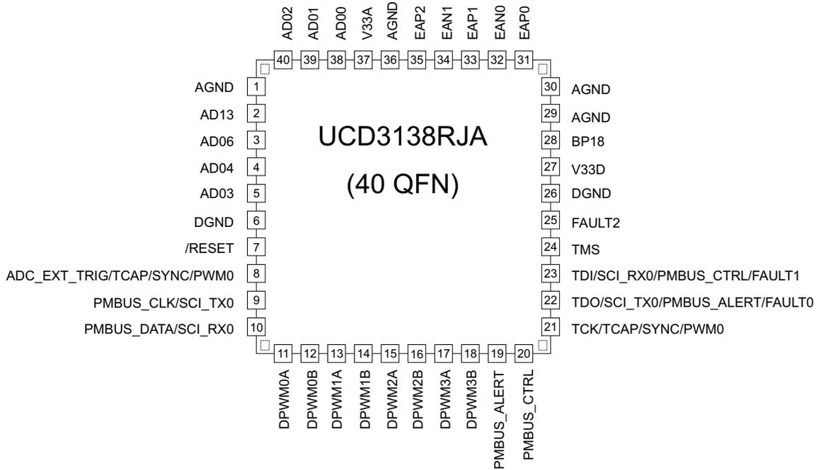
NOTE: The RJA package has thicker package height compared to the RMH package. There are also four corner pins on the RJA package. These features help to improve solder-joint reliability. The corner anchor pins and thermal pad should be soldered for robust mechanical performance and should be tied to the appropriate ground signal.
