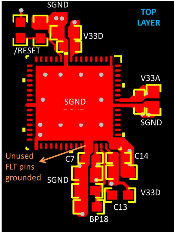
图 12-13. UCD3138 and UCD3138064 64 Pin Layout Top Layer
