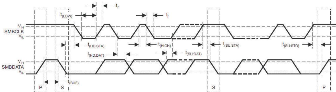
图 8-1. I<sup>2</sup>C/SMBus/PMBus Timing Diagram
