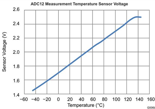
**图 8-9. ADC12 Measurement Temperature Sensor Voltage vs Temperature**
