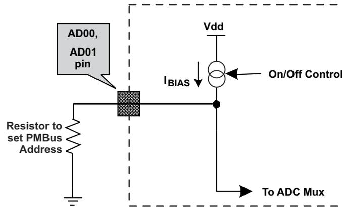
图 9-13. PMBus Address Detection Method
