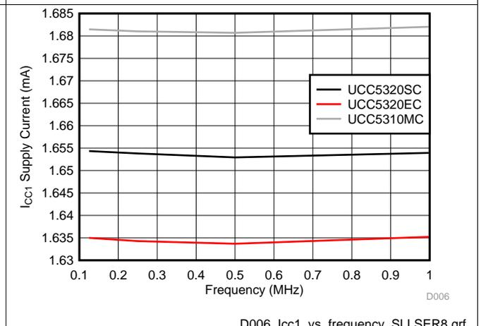
图 14.  $I_{CC1}$  Supply Current vs Input Frequency
