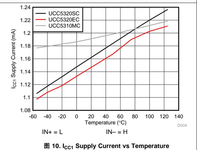
图 10.  $I_{CC1}$  Supply Current vs Temperature
