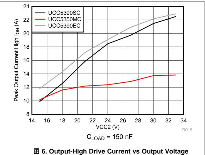
图 6. Output-High Drive Current vs Output Voltage
