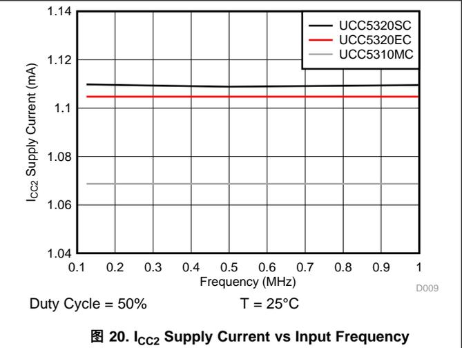
图 20.  $I_{CC2}$  Supply Current vs Input Frequency
