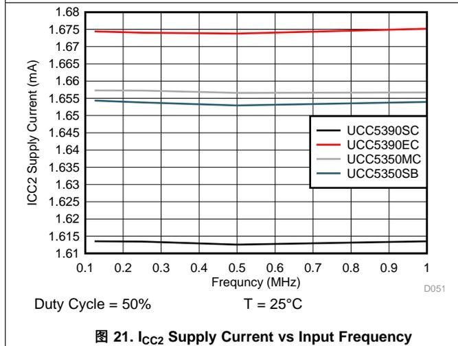
图 21.  $I_{CC2}$  Supply Current vs Input Frequency
