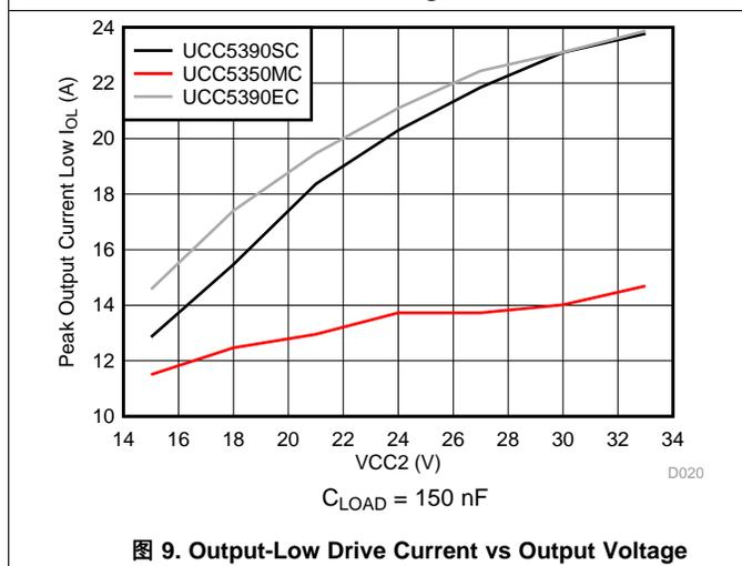
图 9. Output-Low Drive Current vs Output Voltage
