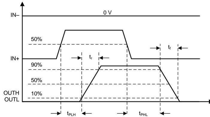
图 42. OUTH and OUTL Propagation Delay, Noninverting Configuration
