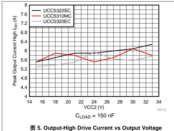
图 5. Output-High Drive Current vs Output Voltage
