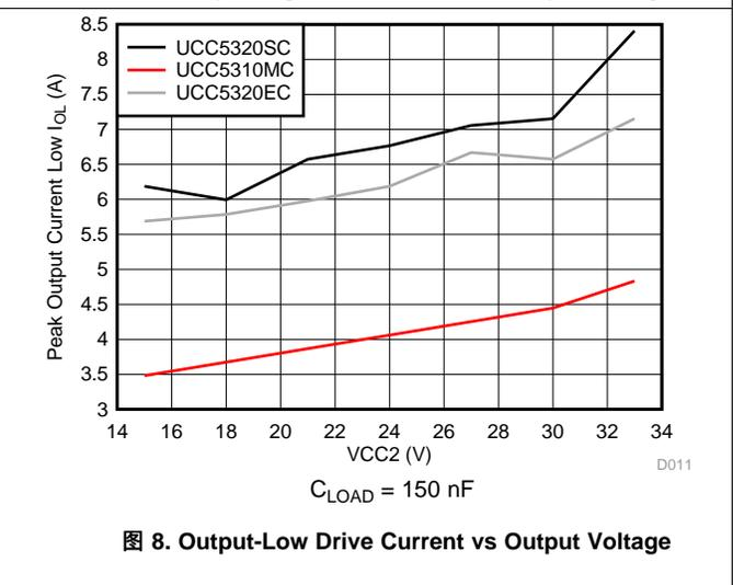
图 8. Output-Low Drive Current vs Output Voltage
