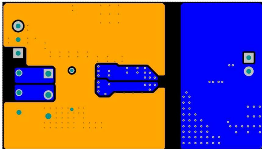
图 65. Bottom-Layer Traces and Copper (Flipped)
