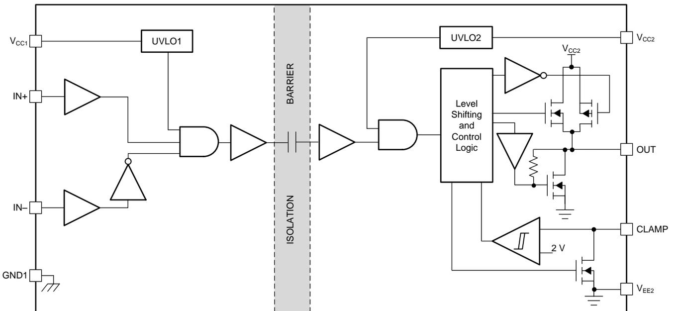
图 50. Functional Block Diagram — Miller Clamp (UCC53x0M)
