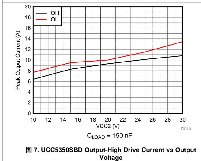
图 7. UCC5350SBD Output-High Drive Current vs Output Voltage
