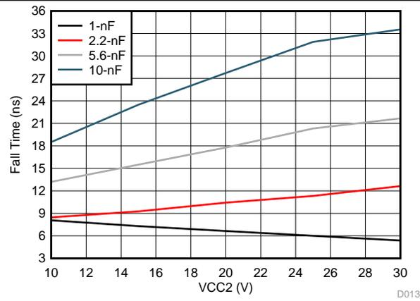
图 41. UCC5350SBD Fall Time vs  $C_L$  and  $V_{CC2}$
