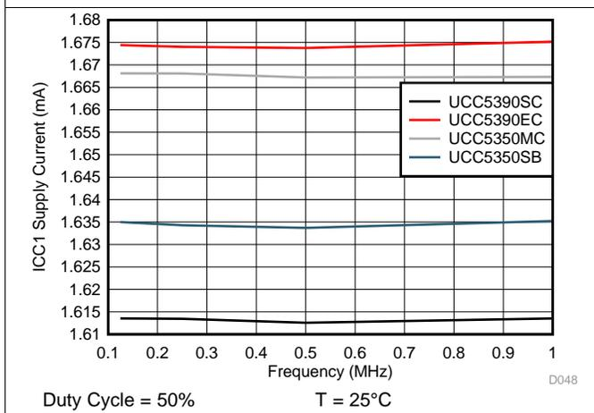
图 15.  $I_{CC1}$  Supply Current vs Input Frequency
