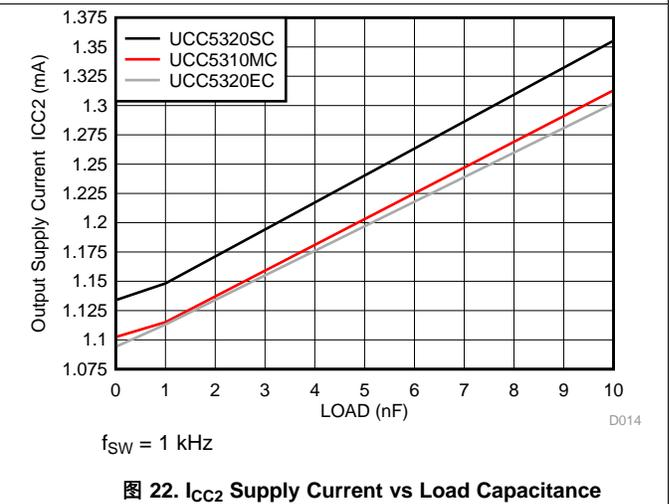
图 22.  $I_{CC2}$  Supply Current vs Load Capacitance
