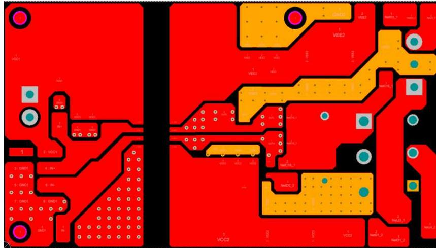
图 64. Top-Layer Traces and Copper
