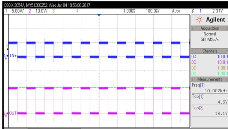
$$V_{CC2} = 20 \text{ V} \quad V_{EE2} = \text{GND} \quad f_{\text{SW}} = 10 \text{ kHz}$$
