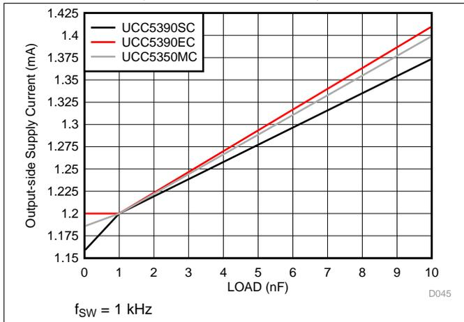
图 23.  $I_{CC2}$  Supply Current vs Load Capacitance
