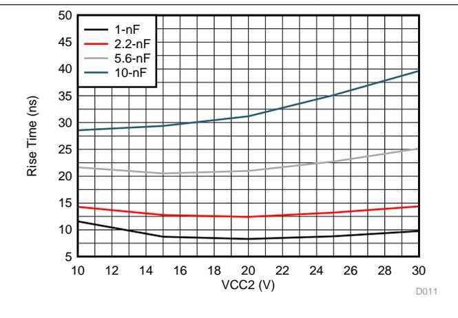
图 38. UCC5350SBD Rise Time vs  $C_L$  and  $V_{CC2}$
