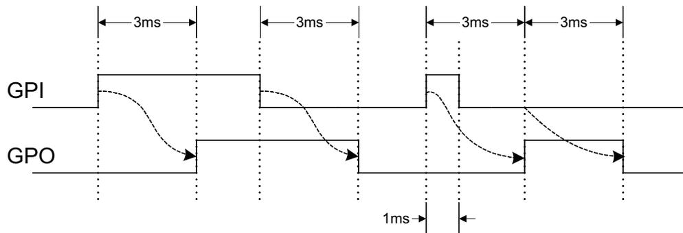
**Figure 21. GPO Behavior When Ignoring Inputs During Delay**
