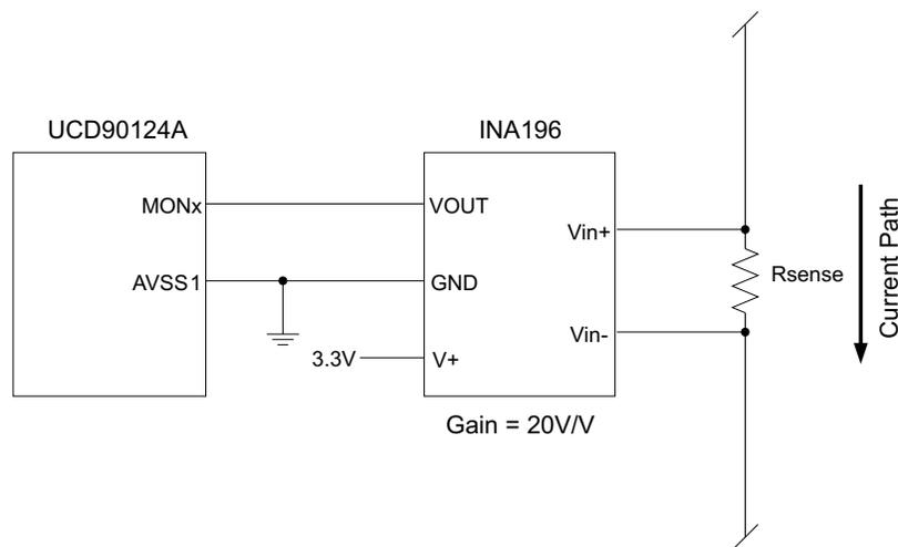
**Figure 13. Current Monitoring Circuit Example Using the INA196**
