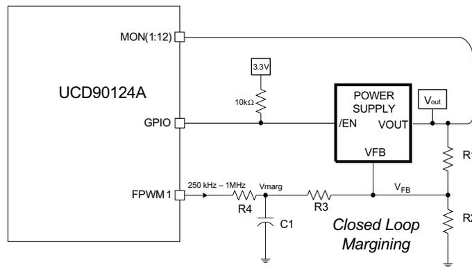
Figure 24. Closed-Loop Margining
