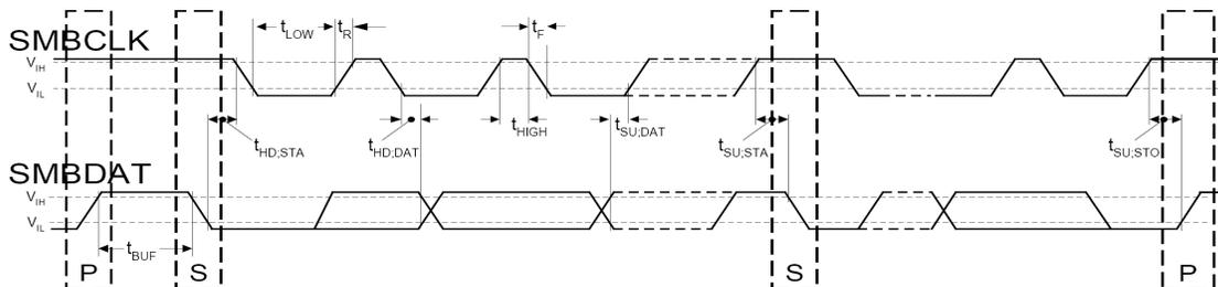
Figure 1. I<sup>2</sup>C/SMBus Timing Diagram
