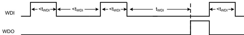
**Figure 32. Timing of GPIOs Configured for Watchdog Timer Operation**
