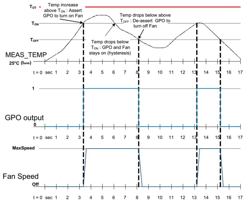
Figure 28. Hysteretic Temperature Control for 2- or 3-wire Fans
