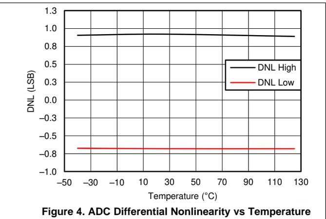
Figure 4. ADC Differential Nonlinearity vs Temperature
