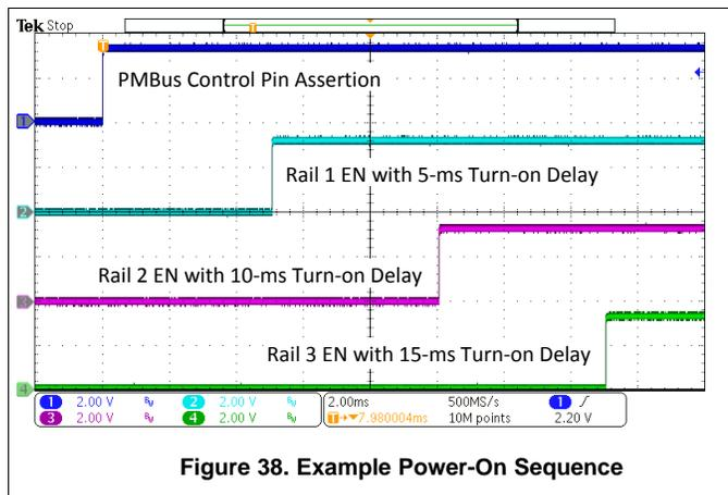
Figure 38. Example Power-On Sequence
