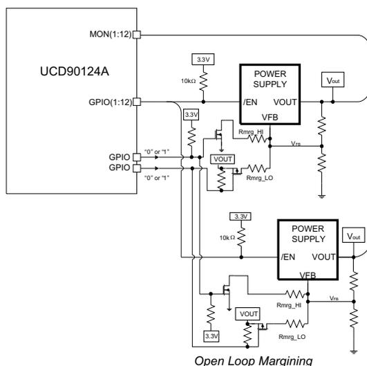
Figure 23. Open-Loop Margining
