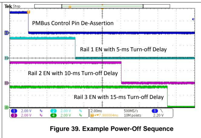
Figure 39. Example Power-Off Sequence
