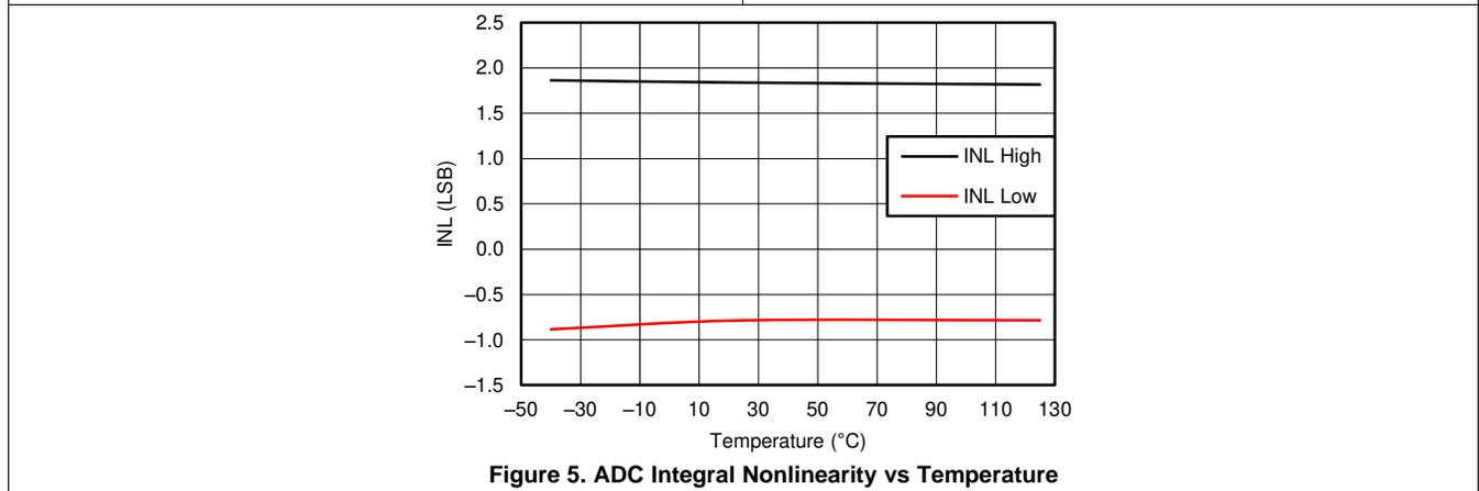
Figure 5. ADC Integral Nonlinearity vs Temperature
