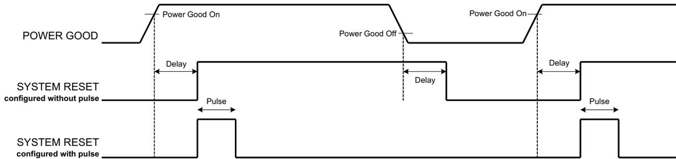
Figure 30. System Reset with and without Pulse Setting
