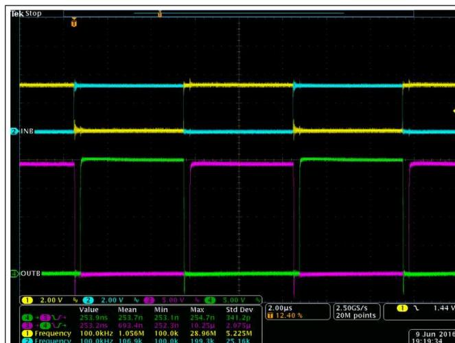
Figure 41. Bench Test Waveform for INA/B and OUTA/B
