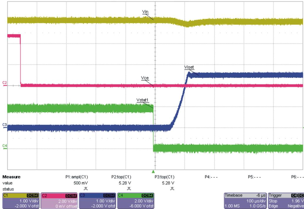
Figure 3. Charge Enable Power-Up Sequence ( $\overline{CE}$  = High-to-Low)
