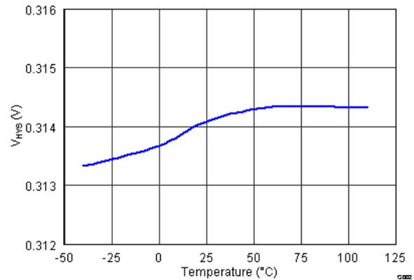
Figure 7-2. Hysteresis V<sub>HYS</sub> vs. Temperature
