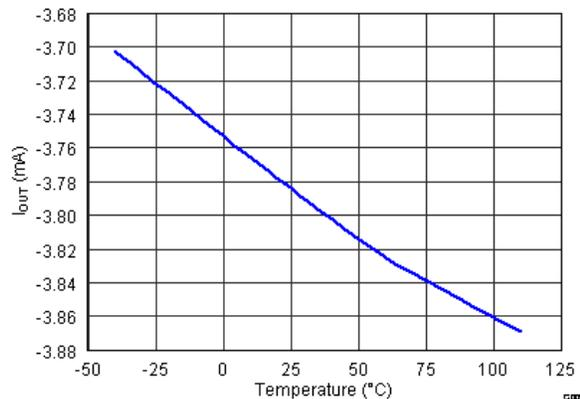
Figure 7-5. Output Current I<sub>OUT</sub> vs. Temperature
