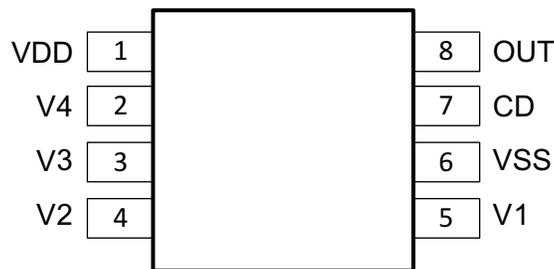
**Figure 6-1. DPJ Package 8-Pin WSON Top View**
