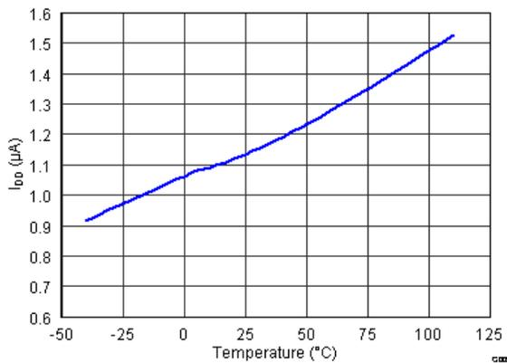
Figure 7-3. I<sub>DD</sub> Current Consumption vs. Temperature at V<sub>DD</sub> = 16 V
