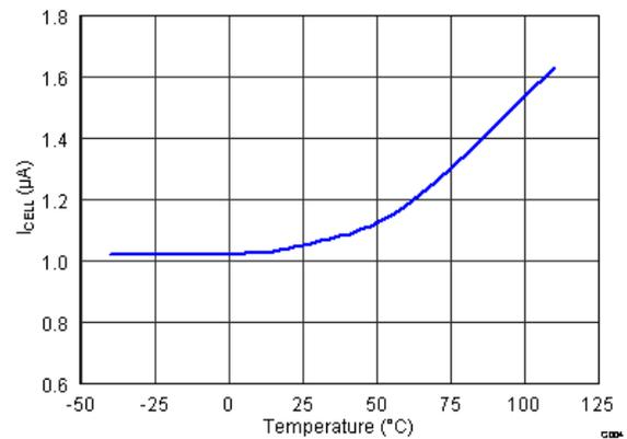
Figure 7-4. I<sub>CELL</sub> vs. Temperature at V<sub>CELL</sub> = 9.2 V
