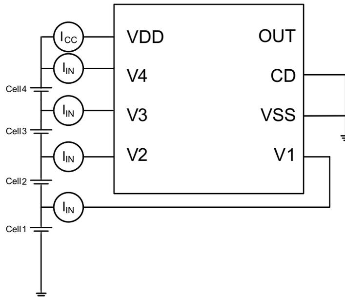
**Figure 8-4. Configuration for IC Current Consumption Test**
