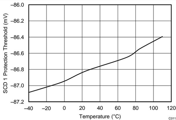
图 39. Short Circuit Discharge 1 Protection Threshold Vs. Temperature
