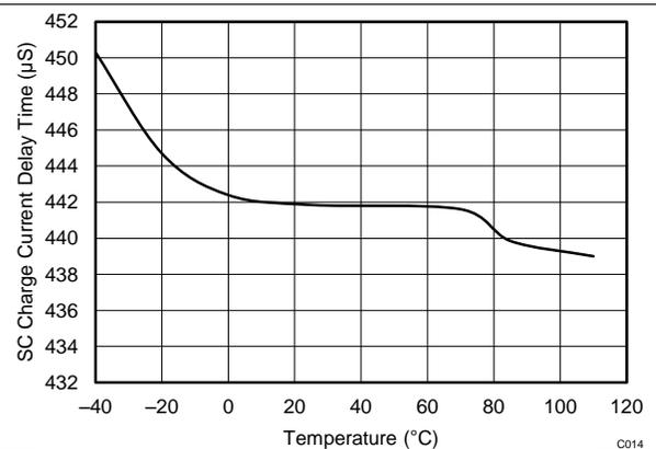
图 42. Short Circuit Charge Current Delay Time Vs. Temperature
