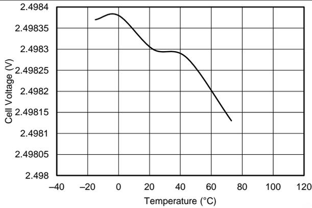
图 17.  $V_{CELL}$  Measurement at 2.5-V vs. Temperature
