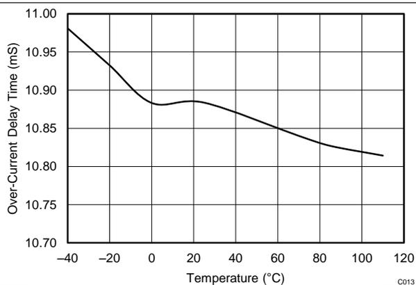
图 41. Overcurrent Delay Time Vs. Temperature
