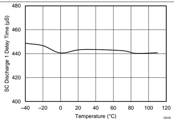
Threshold setting is 465 µs (including internal delay).
