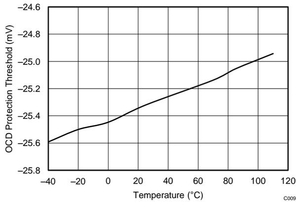
图 37. Overcurrent Discharge Protection Threshold Vs. Temperature
