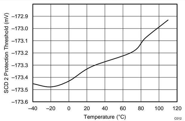
图 40. Short Circuit Discharge 2 Protection Threshold Vs. Temperature
