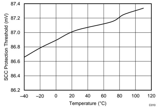
图 38. Short Circuit Charge Protection Threshold Vs. Temperature
