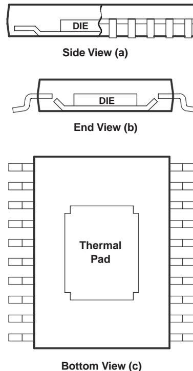
**Figure 20. Views of Thermally Enhanced PWP Package**
