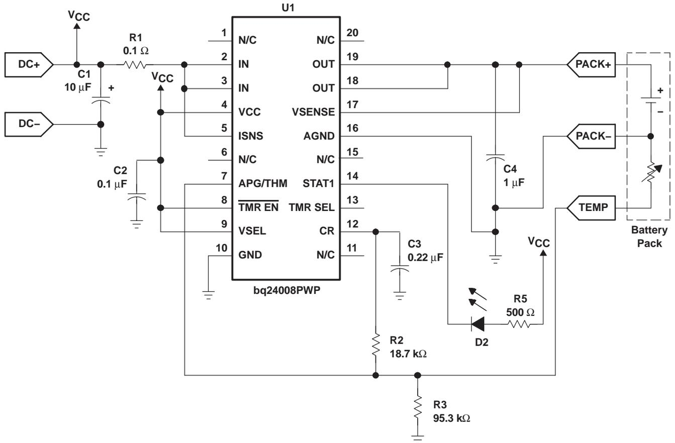
Figure 12. Single-Cell Li-Ion/Li-PoI Charger With Safety Timer Disabled
