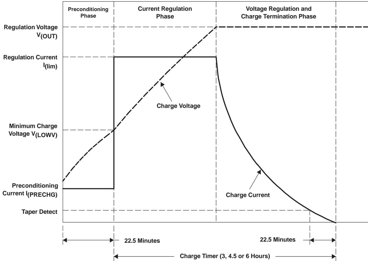
**Figure 13. Typical Charge Profile**
