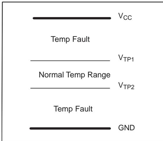
**Figure 17. Temperature Threshold**
