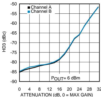
Figure 9. Third Order Harmonic Distortion vs Attenuation
