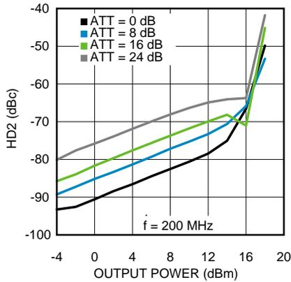
Figure 13. Second Order Harmonic Distortion at 200 MHz
