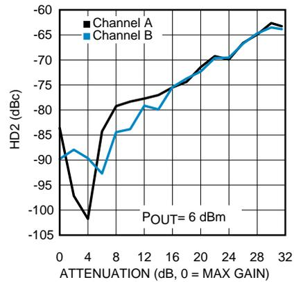
Figure 8. Second Order Harmonic Distortion vs Attenuation
