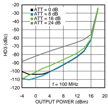
Figure 12. Third Order Harmonic Distortion at 100 MHz
