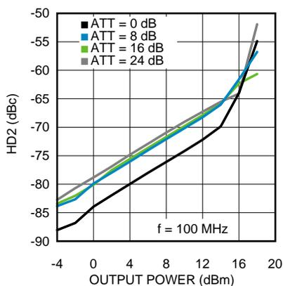
Figure 11. Second Order Harmonic Distortion at 100 MHz
