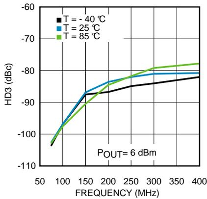
Figure 7. Third Order Harmonic Distortion vs Frequency
