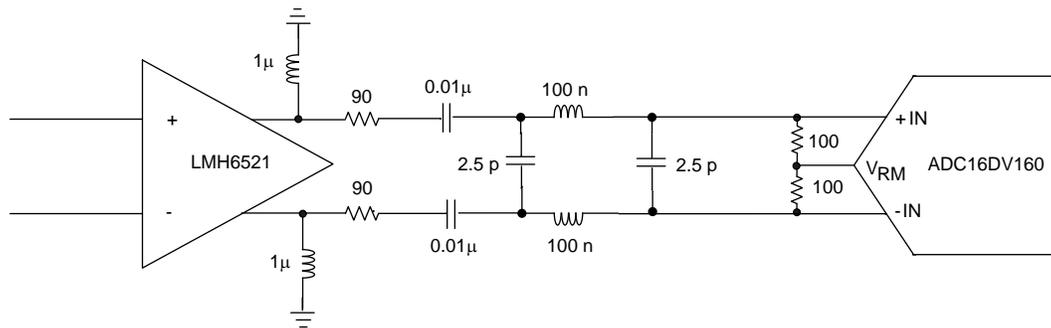
**Figure 40. Filter Schematic**
