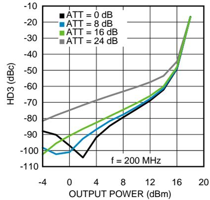
Figure 14. Third Order Harmonic Distortion at 200 MHz
