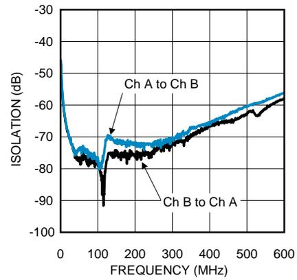
**Figure 20. Channel-to-Channel Isolation**
