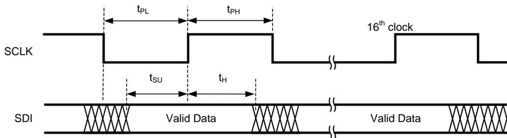
Figure 32. Write Timing, Data Written to SDI Pin
