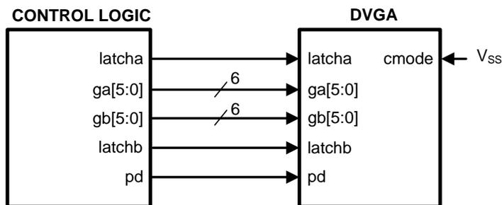
Figure 26. Parallel Mode Connection for Fastest Response
