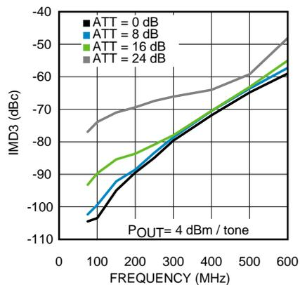
Figure 6. Third Order Intermodulation Products vs Frequency
