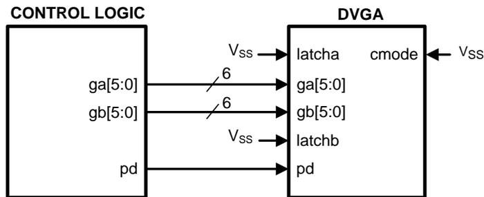
Latch pins tied to logic low state
