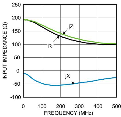
**Figure 21. Input Impedance**
