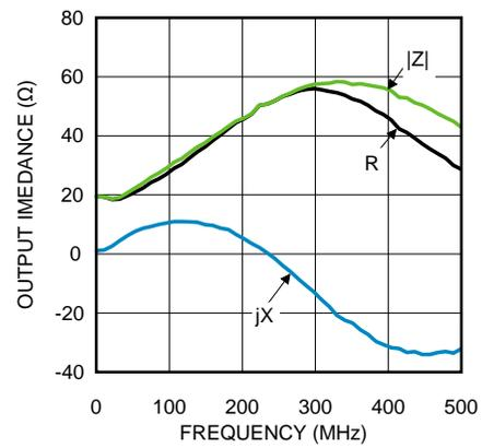
**Figure 22. Output Impedance**
