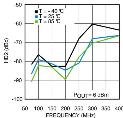
Figure 10. Second Order Harmonic Distortion vs Frequency
