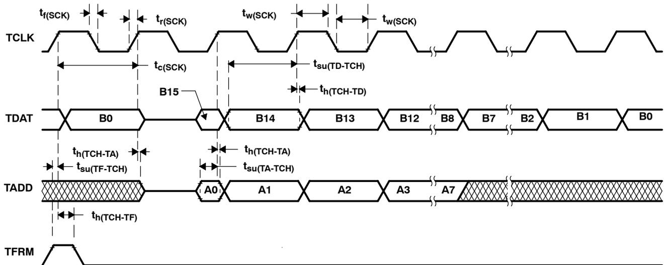
Figure 17. Serial-Port Receive Timing in TDM Mode
