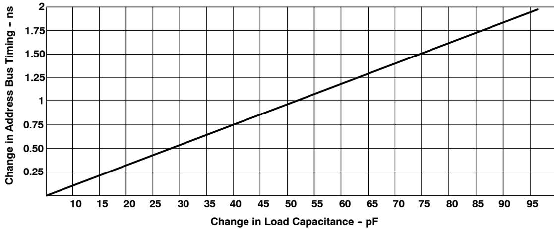
Figure 8. Address Bus Timing Variation With Load Capacitance
