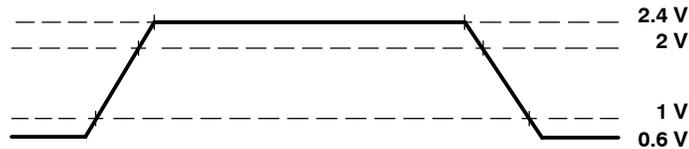
Figure 2. TTL-Level Outputs
