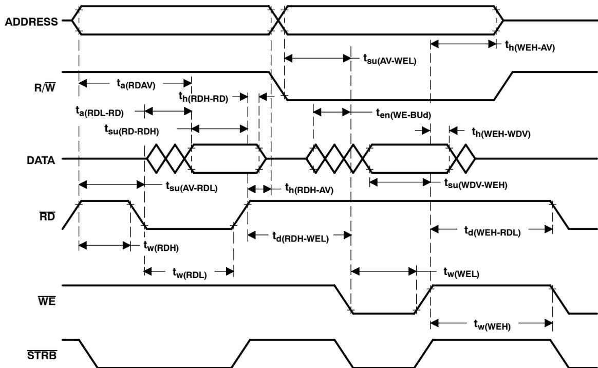
NOTE A: All timings are for 0 wait states. However, external writes always require two cycles to prevent external bus conflicts. The above diagram illustrates a one-cycle read and a two-cycle write and is not drawn to scale. All external writes immediately preceded by an external read or immediately followed by an external read require three machine cycles.
