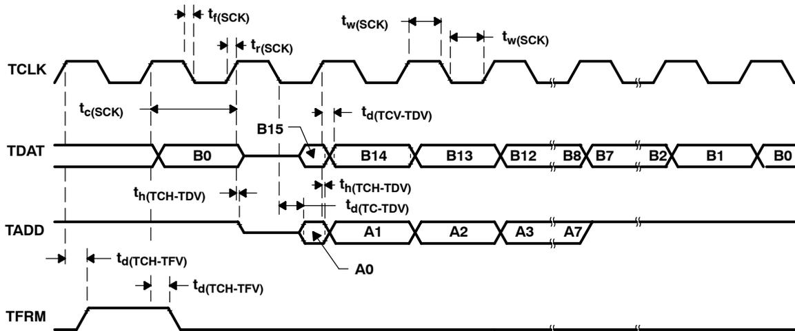
Figure 18. Serial-Port Transmit Timing in TDM Mode
